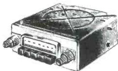
If your CB rig or car radio is transistorized you may feel that you are picking up more noise than you had with tube equipment. This is solved by connecting a special 1000 ufd capacitor to the ignition coil. Ask your auto supplier to get you a
