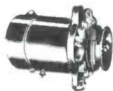
Generators do what their name implies, they generate. They are caused to generate by the action of the motor. Their function is to replace the battery's electricity which is expended in the operation of your vehicle. Generators cause a whining interference in CB receivers, and sometimes the CB rig draws so much current from your vehicle's electrical system that the poor old generator never seems to replace a sufficient amount of juice in the battery. Result? Dead battery.
