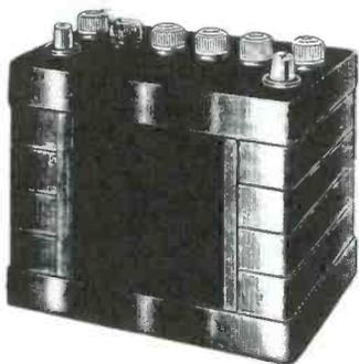
The terminals tend to get a bit corroded, and this impedes the battery's functioning. Use something like "Battery Tru-Rinse" (about 16 oz. for \$1). This will clean off all acid and corrosion with a minimum of work. Check your local auto supply shop for this product.
