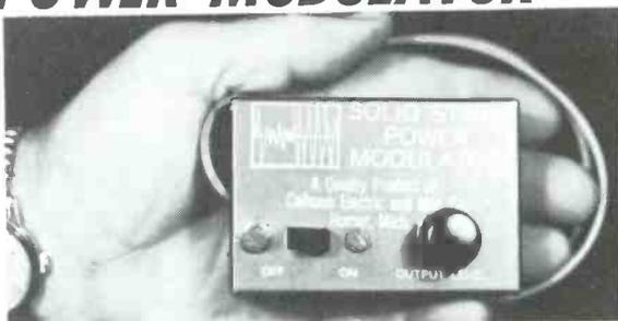
The Solid State POWER MODULATOR is a transistorized audio preamplifier that utilizes the non-linear characteristics of solid state devices to provide a clipper-compressor action which increases the average modulation power of a transmitter.
