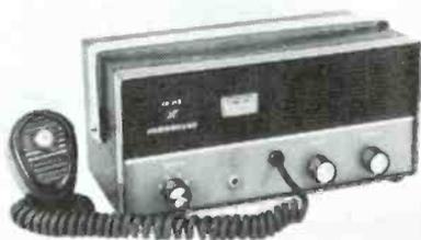
A low cost CB rig was just announced by Hammarlund Manufacturing Company, Inc., 73-88 Hammarlund Drive, Mars Hill, N. C. Dubbed the CB-212 by Hammarlund, it provides 6 fixed transmit/receive channels, a 117VAC/12VDC power supply, ½ uv sensitivity, adjustable squelch, a panel meter and electronic switching. More details from Hammarlund if you write.
