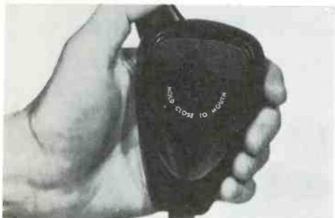
A new lightweight noise-cancelling carbon microphone has been designed by Roanwell Corp., 180 Varick St., New York, N. Y. The RM-515 will cancel an average of 18 db of ambient noise and it is claimed to have improved intelligibility over other available comparable units. Frequency response is 300 to 3.5 kc/s, and it has a PTT button.
