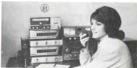
Here's a monitoring station set up for maximum efficiency. On the left (top to bottom) the channel 9 unit (in this case a Pearce Simpson GUARDIAN 23), a Regency MR-10 high frequency police receiver, and a Regency Flight Monitor; on the right is a USL Contact 23 transceiver atop a Lafayette HE-80 communications receiver. At the far right, our cover girl, Susan Henriksen.
