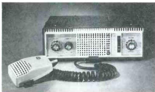
channels; dial marked in both channel numbers and frequency
