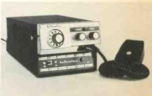
The CB-12 shown mounted on the P-12 base-station pedestal AC power supply on which channel-identification write-in labels are provided.
