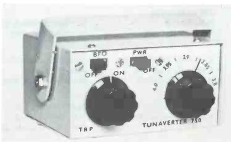
The "Tunaverter," sold by Herbert Salch & Co., has a novel feature—it is tunable. Most converters must be tuned on the broadcast receiver dial.
