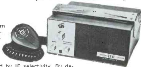
through a crystal bandpass filter. A smooth, adjustable squelch maintains silence when no incoming signal is present. For maximum intelligibility, a built-in 3x5 front-facing speaker is employed. There are provisions for an external speaker and instant conversion to public address via an optional adaptor.
