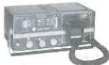
The CB-9 is a six channel CB Transceiver, ready to operate either base AC or mobile 12 VDC, with all power cords and mounting bracket. It uses a new all-electronic push-to-talk circuitry. Features the same "drop-down" chassis as the CB-3A. Has built-in "S" meter and Receiver Variable Tuning for all channel reception plus a spotting switch. Accommodates CB-3A accessories. CB Net \$129.95
