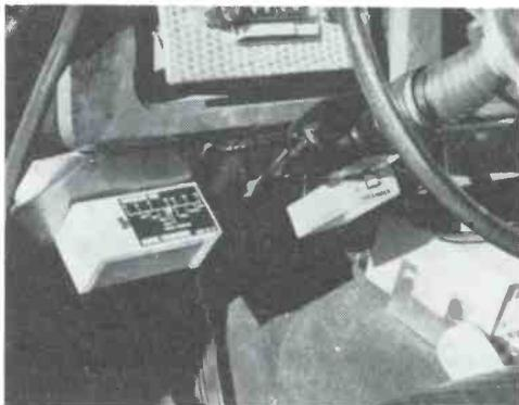
Photo of a complete converted mobile unit. On the left is a Hartman marine converter, in the center a Sentry Electronics police model, and on the right an International Crystal unit for aeronautical frequencies. These units are top-notch and can be recommended highly from personal experiences with them. A Crescent Electronics unit is in use at the base station.
