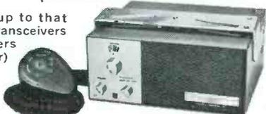
The transmitter utilizes full legal transmitter input (5-watts) with a special high efficiency RF output amplifier, clipped and filtered audio (speech booster) for top talk power (100% modulation). Both units have a built-in power supply for 12VDC (negative ground) mobile operation, mobile
