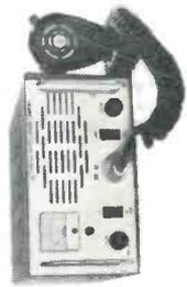
**BB-30:** For business, commercial, and industrial use, the BB-30 is unsurpassed for rugged dependability and performance. 50 watts. Carrier-controlled modulation for constant 100% modulation. 27-36 MC, 12/115 V. ----- \$249.50 Net.
