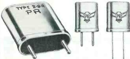
Supplied in all 23 assigned frequencies. Be sure to specify channel desired, with name of manufacturer and model of equipment. Type Z-9R Crystals have .486" pin spacing; .050" pin diameter; .758" height, above pins; width .720" and depth .309". Z-13 Crystals have .192" pin spacing; .040" pin diameter; .530" height above pins; width .402" and thickness .150". Z-13P Crystals are same as Z-13 except for having .017" wire leads instead of pins.
