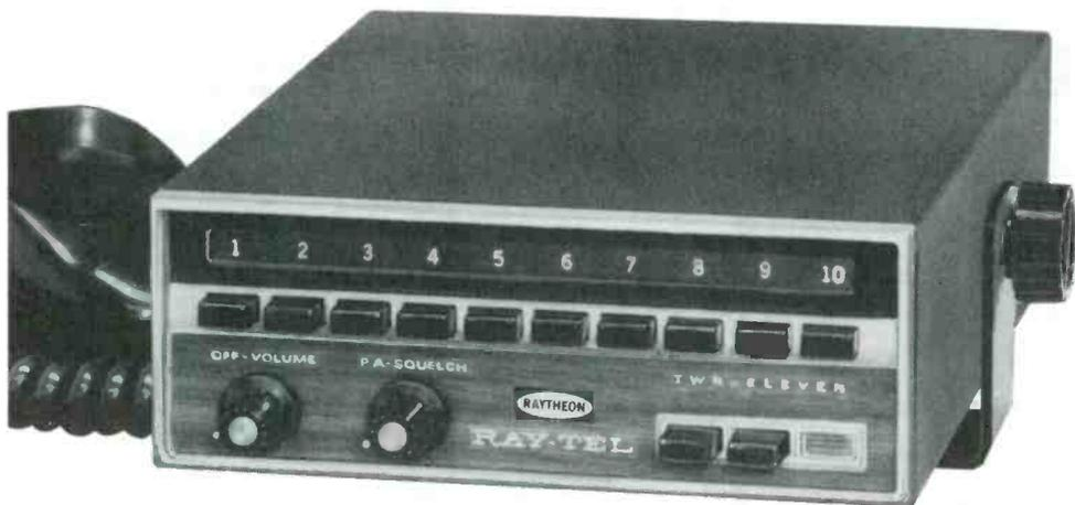
TWR-11 is entirely solid-state—ideal for mobile with direct 12V DC operation, exceptionally low current drain and conveniently small size. But place it on the accessory pedestal 115V AC power supply—connect—and you have an outstanding base station. Distinctive too with woodgrain paneling accented by polished chrome and complemented by black channel-change push-buttons.
