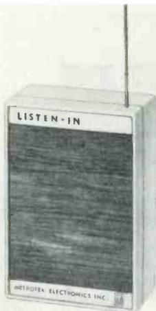
The folks at Metrotek Electronics, subsidiary of Regency Electronics, Inc., 7900 Pendleton Pike, Indianapolis, Ind. 46226, have come up with a pocket sized converter called the "Listen-In." This features crystal controlled operation on any frequency from 25 to 175 mc/s, feeding the received signal into any broadcast radio without any direct electrical connection. Two models are available, a single channel set for \$19.95 and a dual channel unit for \$24.95.
