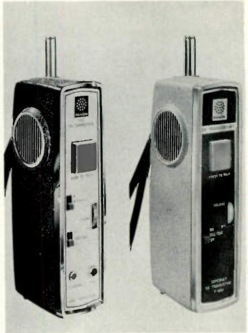
Other advantages include a superheterodyne 'push-pull' receiver with tuned RF amplifier, crystal controlled transmission (crystals supplied for Channel #15) and AGC (automatic gain control) with full modulation. Small in size for handy communications, the units weigh just 9 ozs. each.
