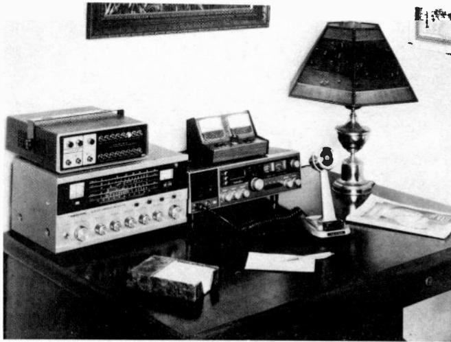
A rather complete installation, including AM/SSB rig (a Realistic Navajo in this case), a scanner, and a communications receiver.
