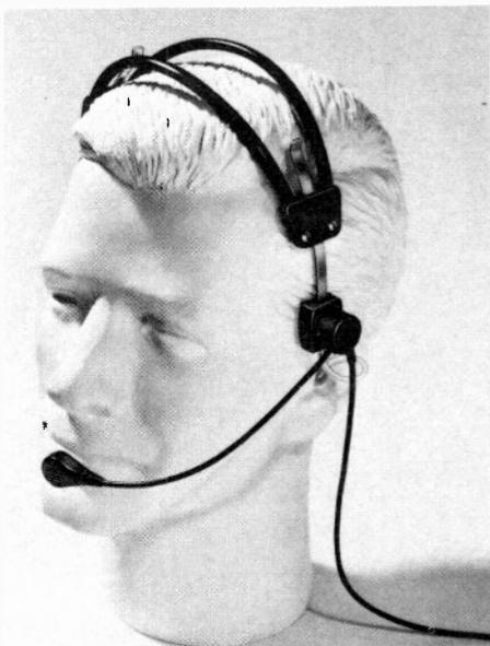
quality. The variable gain can be set for maximum "talk-power" at normal speaking voice. The microphone is mounted on a pivoting boom so it can be placed close to the lips and the unit can be worn over left or right ear. The mike is keyed for transmission by a push-to-talk switch which has a clothing clip for convenient attachment to shirt pocket or jacket lapel.
