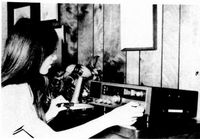
Many sideband rigs come equipped with a "stock" mike of the hand-held type, although most operators prefer to use a desk type for base station operation. It's an easy matter to put a desk type mike on a rig, with power mikes being popular candidates.
