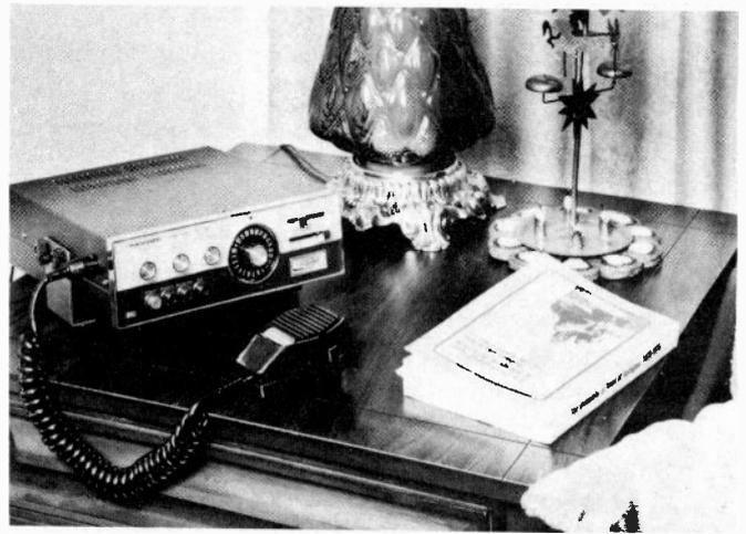
For those who feel that getting a base and mobile SSB rig runs into too heavy an outlay, at least at the start—the option is there to obtain one rig, a mobile unit, which can be used for both base and mobile use. This Realistic TRC-48 is a set which lends itself to dual use—most mobile rigs will require a separate power pack for operation on house current.
