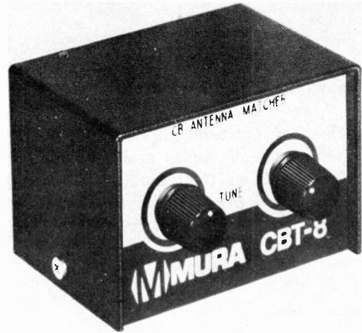
allows the CBer to tune his transmission line to obtain a lower Standing Wave Ratio. A lower SWR means more power transfer from the transceiver to the antenna. "With the CBT-8, the CBer can optimally match his transceiver's output stage to the characteristic impedance of the antenna and transmission line, ensuring maximum power transfer, no matter what CB transceiver or antenna he may use.
