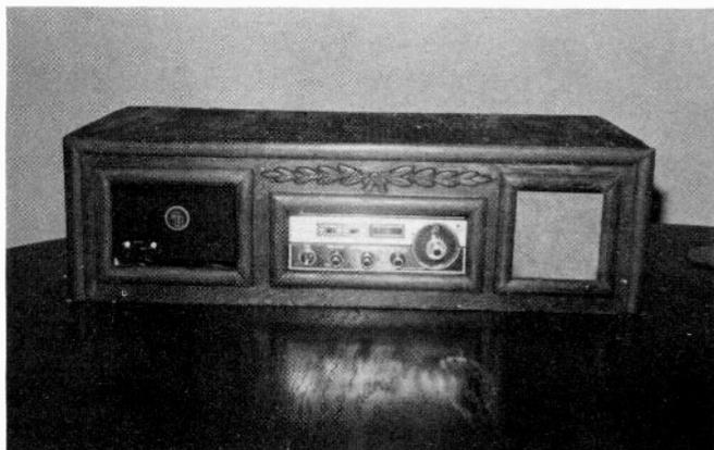
Jan, of San Antonio, Texas, became enthusiastic after reading in CB RADIO/S9 about using a mobile unit combined with a power supply to create a base station, that he took his Cobra 132 out of the mobile
