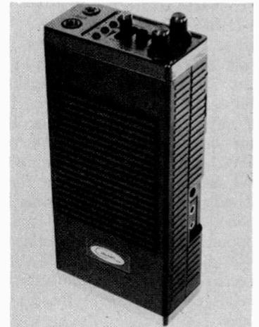
scanners generally exhibit the same sensitivity as conventional mobile unit scanners, but lack a little bit of selectivity that the mobile units generally have greater of. This is why your pocket scanner may not operate at peak efficiency in large cities on an external antennae whereas your mobile scanner does—the pocket scanner simply does not have enough circuitry to offer full selectivity on those tight frequencies.
