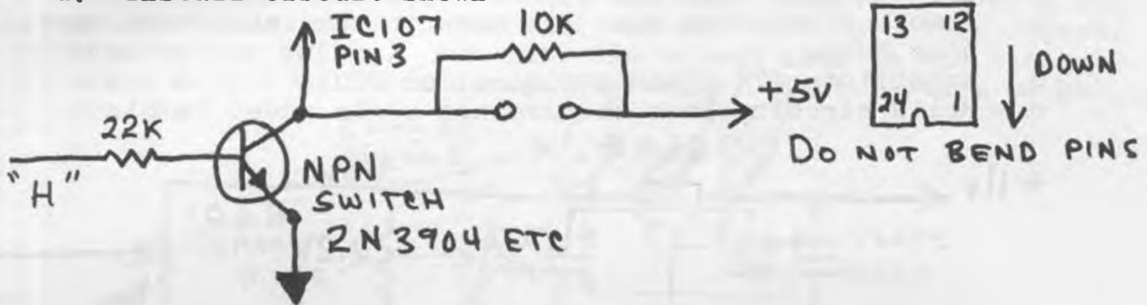
Circuit recognizes greater than 7 (HEX) and switches IC 107/3 low to add 256 to required division.
