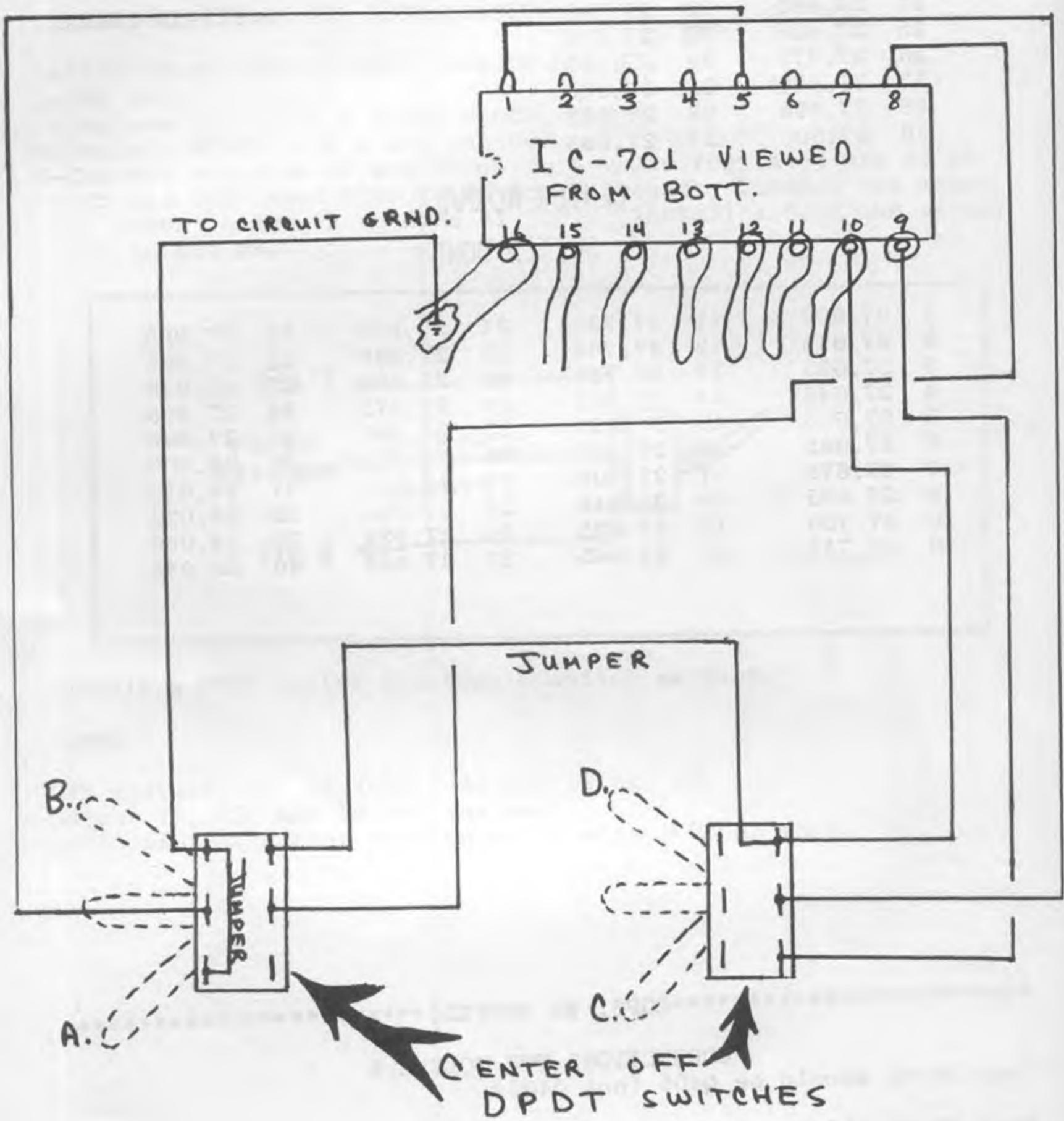
NOTE: PIN #5 and #9 are blank before modification. VCO adjustment is necessary.
