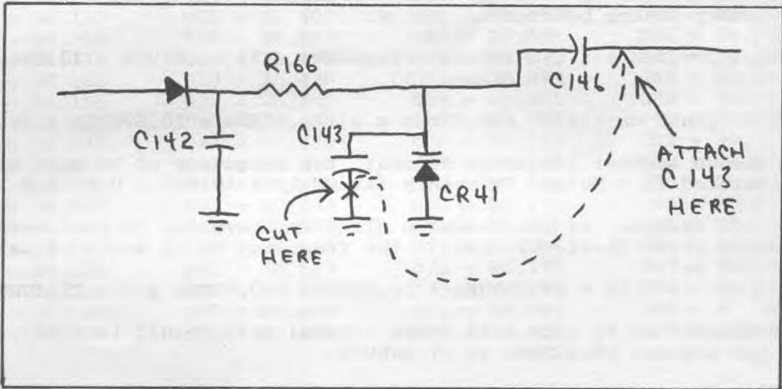
Remove C143 (10pF) and reposition it so it is wired in parallel with C146 (22pF). This will bring the frequency up several KHz. Readjust added coils for exact frequency.
