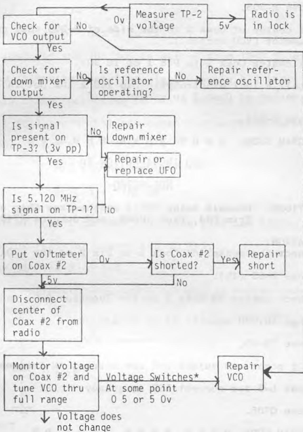
As the VCO is adjusted through the frequency displayed by the UFO, the voltage on Coax #2 should change its logic state.
