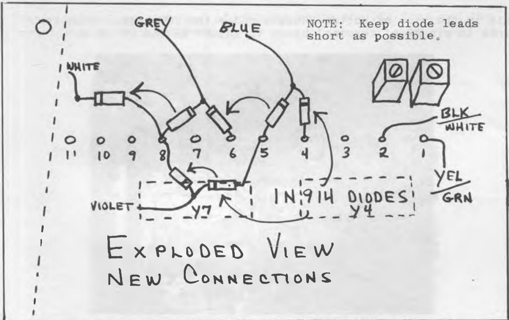
As a note of interest these wires are switched to ground by the channel selector switch to change the left most three digits on the display. Only one wire is used for each position.
