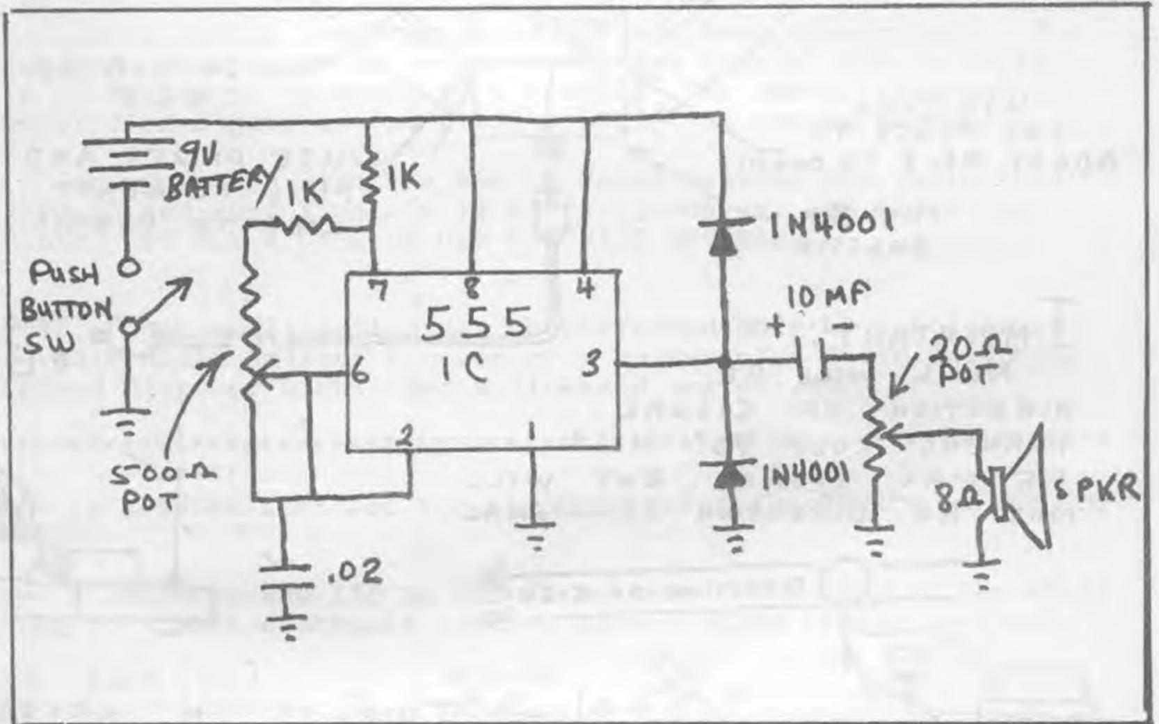
Install all parts on vector board and mount in small box. You may use trim tabs or external controls. If you build two of these units you will have a two tone generator. Mount in the same box. This unit is good for 100HZ to 20 HZ.
