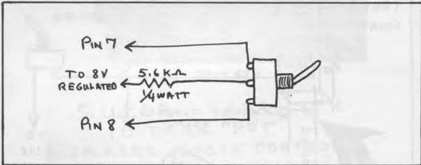
Install a SPDT Center Off toggle switch as show.
