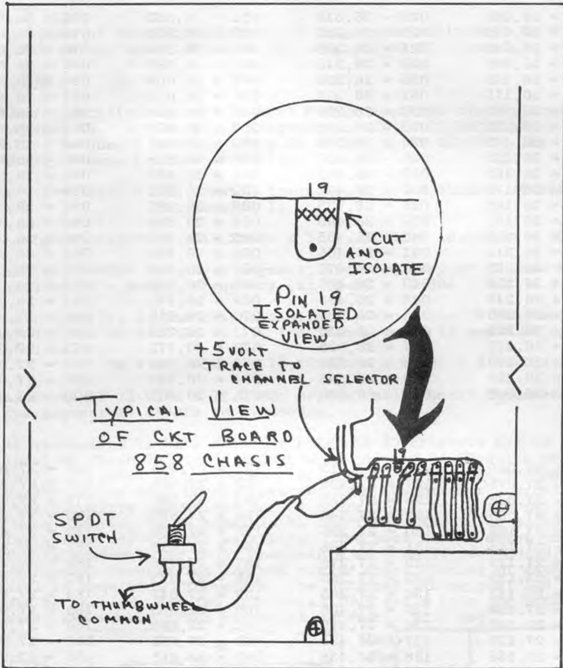
NOTE: You may use existing switch on radio. BE CAREFUL - THIS CAN GIVE YOU TROUBLE IF YOU ARE NOT USED TO USING AN EXISTING N.B. SWITCH ETC. A MINI TOGGLE WILL DO JUST FINE.
