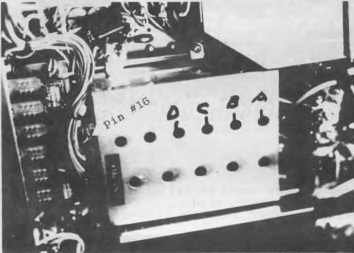
Do not remove cover of VCO unit to adjust. Make the adjustments with a small non-metallic tool.
