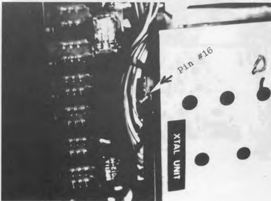
4-Remove counter box in back of display unit. The PLL unit must be removed first to allow the counter unit to be removed. Notice the colored wires soldered in the circuit board next to the two integrated circuits Y7 and Y4. Remove the blue, violet, grey, and white wires from the circuit board and re-connect them as shown, using silicon diodes in series.
