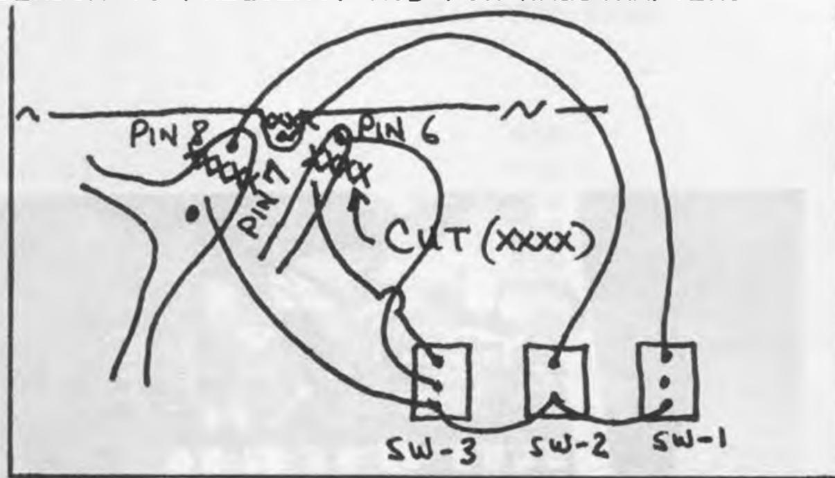
The addition of SW-3 will give: (SW-1 ON, SW-2 OFF, SW-3 ON)
