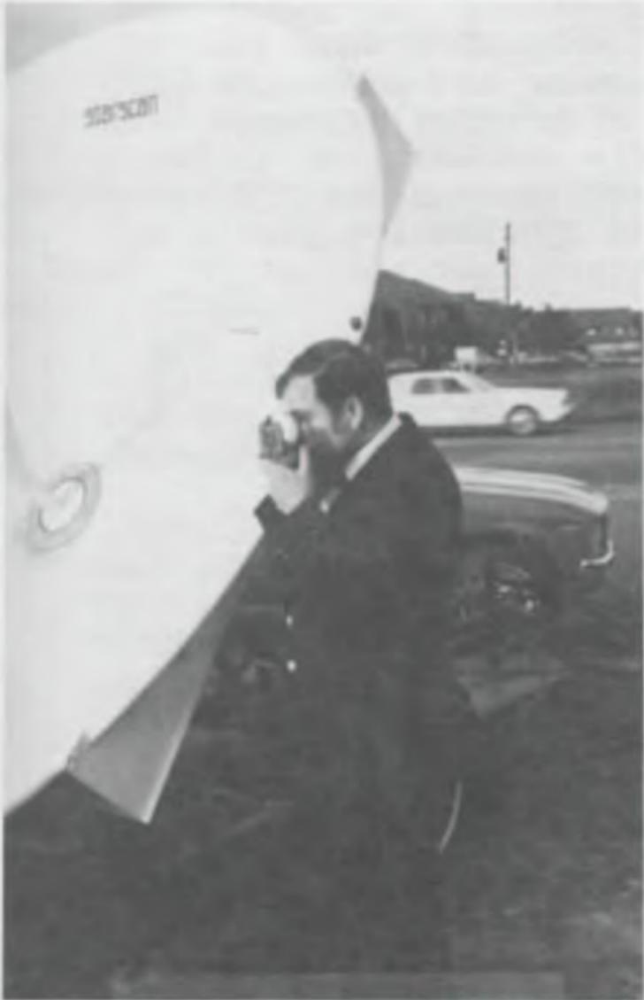
Author, Rod Johnson is shown here using a Brunton handheld transit to locate the SATCOM I bird. Exact azimuth and elevation calculations are required in order to pick up the signals from any satellite. (We'll show you a couple of ways to calculate this in the first volume of Secrets of Satellite TV).
