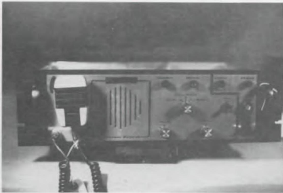
This is the REPCO Repeater, hailed to be one of the finest on the market in its price range. Featuring all modular construction, 100% solid state, time-out timer, automatic transfer AC to DC, and more. Power output is 25 watts.
