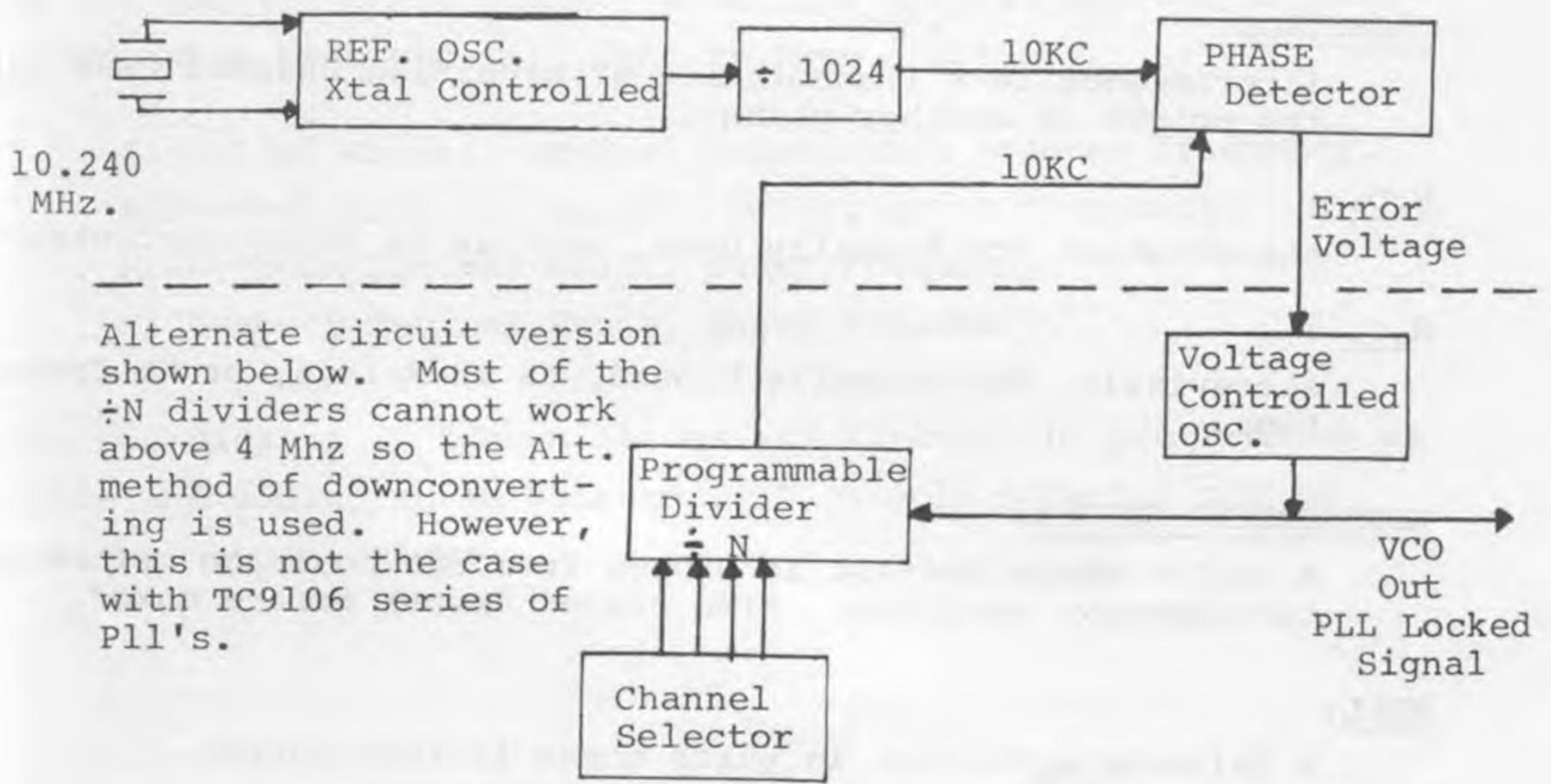
Alternate circuit version shown below. Most of the ÷N dividers cannot work above 4 Mhz so the Alt. method of downconverting is used. However, this is not the case with TC9106 series of Pll's.
