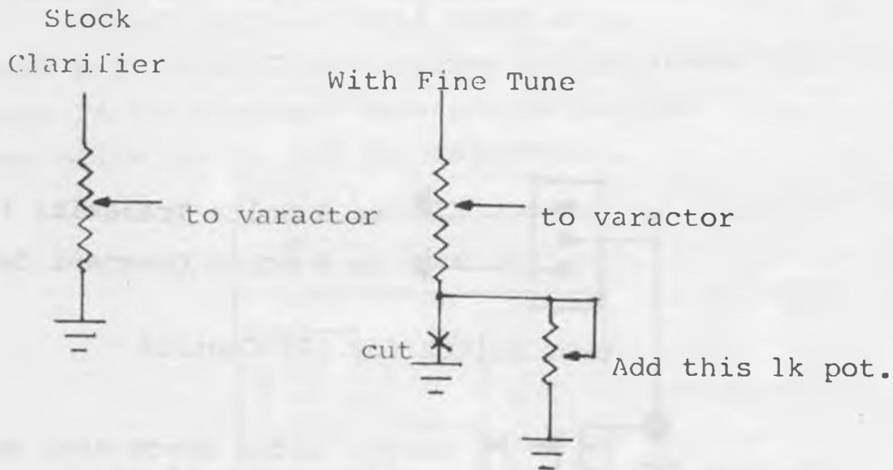
1. Unsolder Clarifier from ground. (sometimes there will be a resistor in series-if so, remove resistor)
