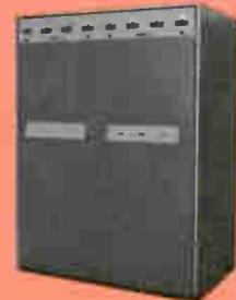
The two tube FM-20 KB offers the modern broadcaster built-in provisions for stereo and SCA. Neutralization is eliminated by the use of grounded grid operation.
