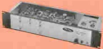
The AEL Model 2203 Stereo Generator has been designed to produce a composite stereo signal that can be fed directly into the audio input of a direct FM Exciter.
