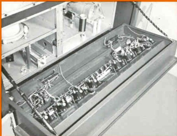
Easy Access Drop-Down Meter and Control Panel
