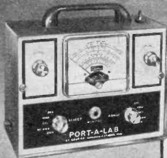
Port-a-Lab Measures SWR, RF Power, Modulation Percent, and Field Strength
