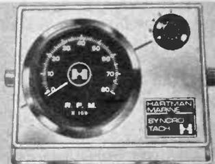
ST-703. Portable wireless tachometer for spark ignition engines—no connections, no installation. Detects engine trouble, determines highest efficiency. Reads 0-8000 rpm with 3% accuracy. On-off sensitivity control. Size, 2x5x6 1/2". With 9-volt battery. Wt., 1 lb.
