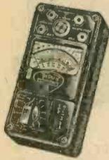
A new and improved instrument built around a sensitive, accurate "Red Dot" Lifetime guaranteed meter. Provides the following scales: 0-10-50-250-1,000-5,000V. A.C. DC. at 1,000 ohms per volt; 0-10-100-500 M.A. D.C.; 0-300-250,000 ohms. Higher resistance readings may be obtained with external battery. A compensated copper-oxide
