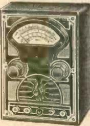
A highly accurate Multitester using a 2,000 ohm-per-volt 5" D'Arsonval meter. Ranges are: 0-5-50-500-1,000 V. D.C. at 2,000 ohms per volt and A.C. at 1,800 ohms per volt; 0-500 microamps D.C.; 0-5-50-500 M.A., D.C.; 0-100-750-75-100 ohms; 0-10 megohms; -12 to +54 DB. in 4 steps; and 4 output inner ranges. Low ohmmeter scale reads 2 ohms at center. Has a complete self-contained power supply. No batteries are required.
