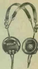
High sensitivity headphones of new piezo-electric design. For Amateurs, Short Wave fans, monitoring, measurement work, etc. Have unusually high impedance and wide frequency response between 60 and 10,000 cycles. These phones are ideal for all applications. When used in circuits carrying direct current, a small blocking condenser is required. Weight including band and cord, only six ounces. One of the finest headsets on the market. Shpg. wt., 2 lbs.
