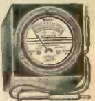
A very popular, pocket-sized test instrument. Ranges are: 0-300 V. D.C. and 0-10,000 ohms. Uses a magnetic vane type meter with 2" dial. Ranges are selected by means of jacks and a plug. The black hard-wood case measures 2 1/4"x2 3/4"x1 1/2". Easily fits in a pocket. Ohmmeter circuit uses 2 self-contained standard dry cells. Supplied complete with 24" polarized leads, test prods, and batteries. Shpg. wt., 1 lb.
