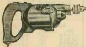
An ideal drill for maintenance and installation work. Made by a leading manufacturer. Husky aluminum casing. Famous "Compo" oilless bearings will give years of smooth operation. Can be used in stand for light grinding and wire brushing. Universal 110-120 volt AC-DC motor operates at 1800 R.P.M. without load; 1050 R.P.M. with full load. Length 12".
