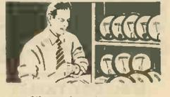
**SERVICE A:** For  $3\frac{1}{2}$ " meters with burned-out or open armatures. We dismantle the entire moving element, revind or replace armature, replace and sharpen the pivots, and polish the jewels. If the armature has been burnt, new hair-springs are installed. The moving element is then reassembled and balanced, and the meter calibrated at three points. Scratched metal cases are carefully refinished. **\$3.75**
