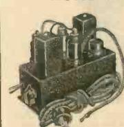
Designed to reduce static and man-made interference. Based on the famous Lamb circuit. Operates with any superheterodyne having an I.F. of 450 to 470 K.C. Silencer supplies its own filament current. Equipped with tube prong for plugging into receiver. Uses 1 each—6K7, 6J7, 6L7, and 6H6 tubes. With instructions. 8 1/4"x5 3/4"x3 1/4". overall. Shpg. wt., 3 lbs.
