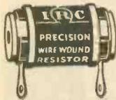
Ideal for use as meter multipliers and shunts. Accuracy within 1%. Values to 500,000 ohms have lug terminals; size: 1"x3/8" dia. Others have knurled nuts; size: 2 1/8"x7/8" dia. Available in odd sizes on special order at cost of next higher value.
