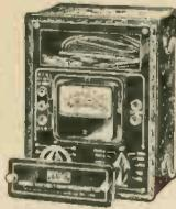
An outstanding Volt-Ohm-Milliammeter for field or shop use. Uses a Triplett Model 326 precision meter. Ranges are 0-10-50-250-500-1,000 V. D.C. and A.C. at 1,000 ohms per volt; 0-1-10-50-250 M.A. D.C.; 0-300-250,000 ohms (25 ohms center scale); 0-250,000
