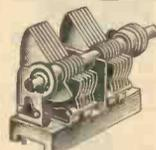
Rigid, high quality two-gang midget condensers, designed especially to provide added efficiency at ultra-high frequencies. Plates are .0225" brass; .0245" air-gap. Overall length behind panel, 3/4".
