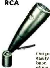
MODEL BK-1A PRESSURE MIKE. High-fidelity "Commentator" pressure microphone designed for broadcast use in AM, FM and TV stations. Rugged, insensitive to wind and mechanical vibration. An excellent microphone for outdoor use where constant handling is necessary. Smooth, extended frequency response of 60-10,000 cps.
