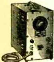
For adjustable, regulated, harmonically neutralized AC. Two outlet receptacles accept variable voltage. One fixed, 115 v.; other variable, 0-130 v. Two panel jacks (for leads) provide additional 0-130 v. output. Outputs can be used simultaneously. Harmonic distortion, less than 3%. Regulating response time, 1.5 cycles or less. Sizes: 50105 is 12 1/2 x 7 1/2 x 4 1/2"; 50106 is 13 1/2 x 7 1/2 x 4 1/2". For 95-125 volts, 60 cycle AC.
