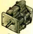
**Fig. B. 365 Mmf Capacitors.** Compact TRF variables. Have trimmers on side of frame. Outer rotor plates are slotted for tracking adjustment. Tapped holes in frame provide secure mounting. Range: 10 to 365 mmf. Shaft diameter,  $\frac{1}{8}$ ". 2 gang:  $2\frac{1}{2} \times 1\frac{1}{2} \times 1\frac{1}{4}$ ". 3 gang:  $3\frac{1}{2} \times 1\frac{1}{2} \times 1\frac{1}{4}$ ". Shpg. wt., each, 6 oz.
