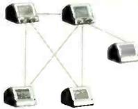
A combined system of Masters and Subs. Ideal for installations requiring several Masters in communication with all other stations. Subs can answer any Master but do not originate calls.
