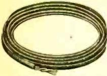
A general purpose, thermoplastic insulated hook-up wire for applications at 1000 volts rms or less. Made to conform to stringent government specifications. Feature high dielectric strength, stability at high temperatures, flexibility at low temperatures and very low moisture absorption. Flame and fungus resistant. Vinyl thermoplastic insulation is virtually impervious to damage from solvents. Nominal diameters: Type 8530, .059"; Type 8524, .064"; Type 8529, .066"; Type 8523, .072".
