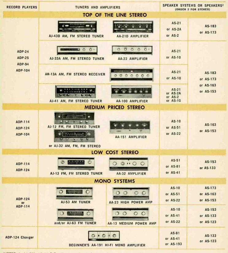
NOTES: 1. AA-100 and AA-21D will operate directly from tape head. All other amplifiers require tape head preamps. 2. Individual speakers must be provided with suitable acoustic enclosures, or home-built to included instructions.
