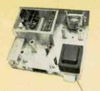
Convenient Chassis Layout Easy access to crystal sockets, shielded final amplifier, lowpass filter. Permits fast, easy assembly.
