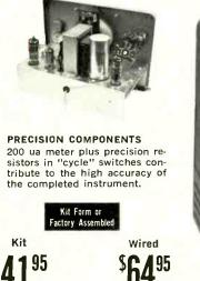
**METERED OUTPUT VOLTAGE.** Generator output is indicated on a large  $4\frac{1}{2}$ " 200 ua meter calibrated in volts and decibles for exact settings to test conditions. Output attenuator operates in steps of 10 db and is calibrated in 8 fullscale meter ranges. A variable output attenuator provides "fine" adjustment on each range, and a slide-switch selects either built-in or external 600 ohm load. Order one of these fine units for your test bench now.
