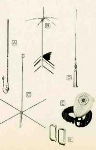
A Model GY-12 Cowl Mount Mobile Antenna, 2 Ibs...\$8.95. 48" fiberglass whip. Patented rocker support for 8-point ground. Complete with 15' RG-58U cable and connector.
