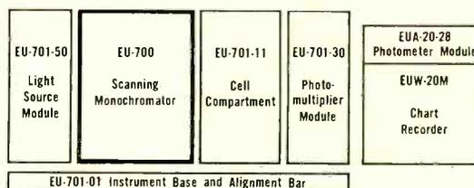
Shown above are illustrations of the modular concept common to all Heath scientific instrumentation. The "700" Monochromator is the basic module of these and of an extensive series of future instruments. And as new techniques are developed, Heath will provide the required modules. The Heath
