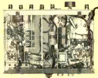
**Compartmentalized Chassis Construction** . . . each function area is shielded for the high stability required at these frequencies.
