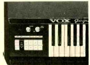
**Separate Bass Output** to connect solo bass to a separate bass channel or amplifier, thus creating a brilliant "stereo" effect. Also allows you to emphasize or keep the bass constant with the bass volume control while changing the treble keyboard volume with the expression pedal.
