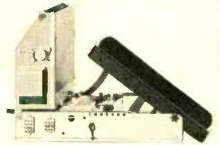
Two All-Transistor Amplifiers . . . one for the Leslie speaker system and the other for the main system . . . deliver a total of 200 watts of peak power. Run cool and collected for long, trouble-free life.
