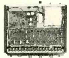
Easy to Build . . . everything but the switches and controls mount on three circuit boards . . . oscillator circuits are shielded.
