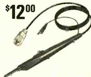
PKW-2 PROBE MINIMIZES CIRCUIT LOADING & SIGNAL DISTORTION . . . designed for scopes with 1 megohm input, such as Heathkit IO-14. Features miniature switch for x1 or x10 attenuation. Impedance in x1 position is 1 meg shunted by 110 pF . . . 10 meg shunted by 20 pF in x10 position. Response is DC to 25 MHz. Max. DC voltage is 600 V. Features spring-loaded clip tip for hands-free operation.
