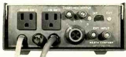
On the rear panel of the Control Unit are the output terminals for the synchronizing pulses to the recorder, a chart-recorder synchro-switch, input terminals and selector switch for external scan rates.
