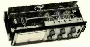
Unitized Construction. Circuit board mounts within the main frame. Cabinet shells are removable for convenient access to calibration controls and battery holders.
