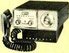
OPERATES "FIXED" . . . with accessory AC power supply GWA-14-1. AC power switching is accomplished through the On-Off Volume control on the transceiver front panel. The GWA-14-1 serves as a handy desk-top base for the GW-14 transceiver, and provides all necessary power . . . requires only one plug-in connection.
