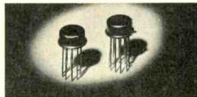
**Integrated Circuits.** Two in the IF amplifier for hard limiting, temperature stability and reliability. Each is only the size of a tiny transistor, yet contains 28 actual parts . . . 10 transistors, 11 resistors and 7 diodes.
