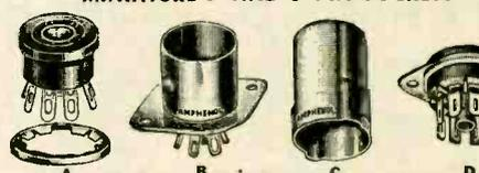
Type A—Miniature retainer ring type sockets mount in "D" shaped or round hole. 3/8" diameter. Types B, D—Miniature 7- and 9-pin sockets. 7-pin sockets mount in 3/8" hole; mounting centers 1/4". 9-pin sockets mount in 3/4" hole; mounting centers 1 1/4". Shielded sockets mount above chassis; unshielded sockets mount below.
