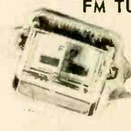
Small, but quite functional, FM tuning meter gives clear center scale indication. Accurate moving vane-type movement has sensitivity of 10,000 ohms per volt from null center to either end of scale. Polarized screw terminals are supplied with solder lugs. Mounts through panel in 1/2" high x 3/4" wide hole with 1-3/16" mounting centers. Extends 3/4" behind panel. Individually boxed with instruction sheet. **\$2.49**
