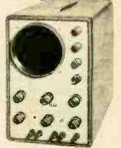
For servicing audio, communications and industrial equipment, including Zener diode calibration and direct access to vert. plates. Vertical amplifier flat from DC to 500kc (-6db at 1mc) and sensitivity is 3.5mv rms/cm. Automatic sync and sweeps continuously variable from 10cps to 100kc in 4 ranges.
