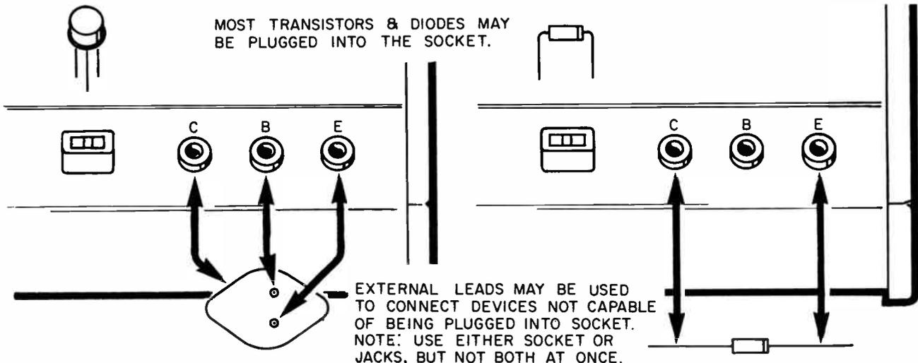
Figure 9. Semiconductor Device Connections to Curve Tracer
