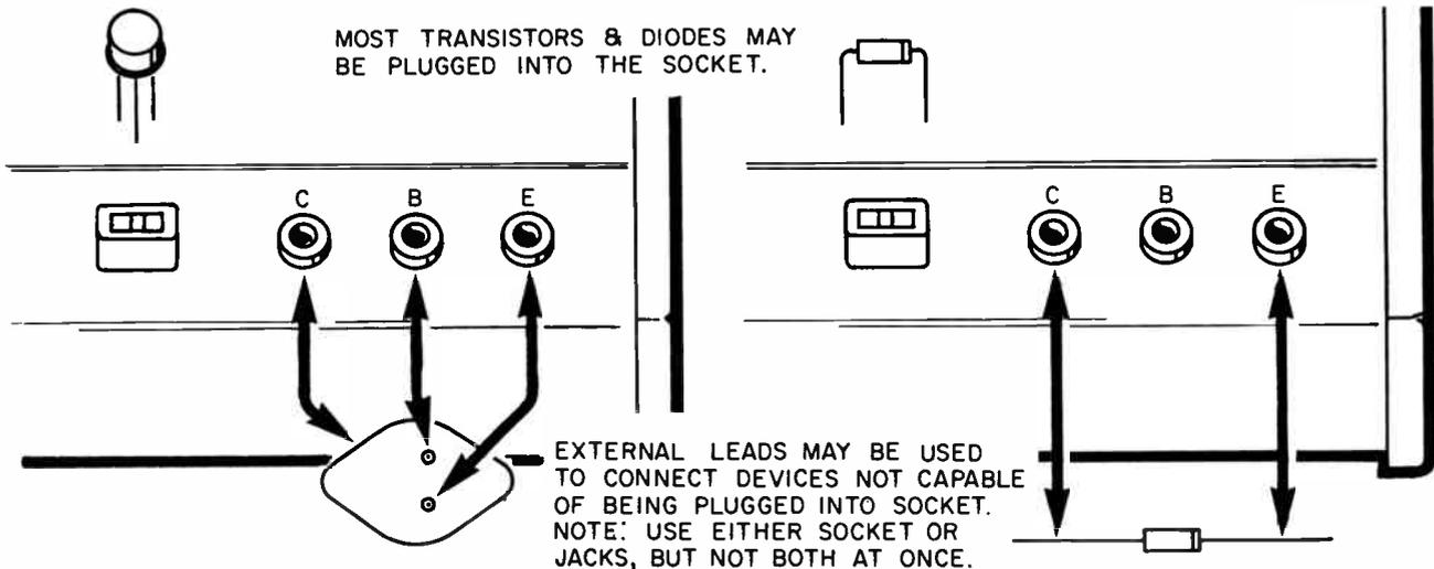
Figure 9. Semiconductor Device Connections to Curve Tracer
