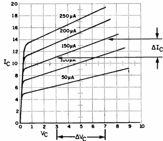
$$h_{oe} = \frac{\Delta I_C}{\Delta V_C} \quad h_{oe} = \frac{3\text{mA}}{4} \quad h_{oe} = .75 \times 10^{-3} \quad h_{oe} = 750 \mu\text{mhos at } I_B \text{ of } 150 \mu\text{A}$$
