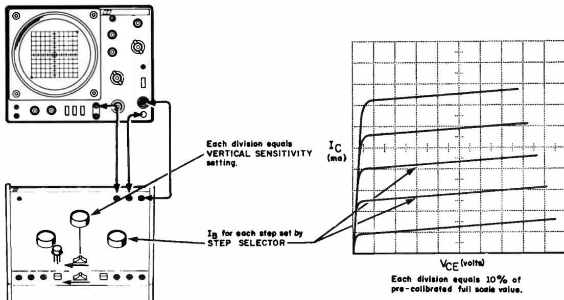
Figure 10. Typical Test of an NPN Transistor
