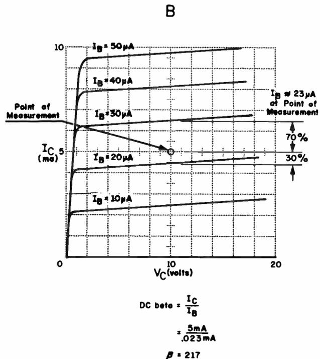
Figure 17. DC Current Gain (DC Beta) Measurement
