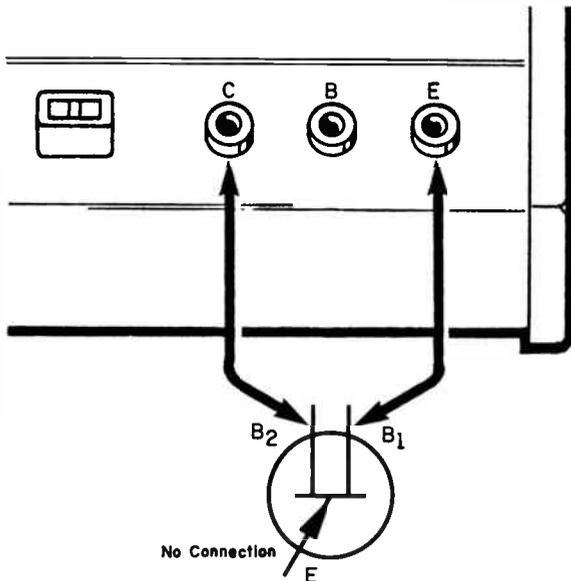
Figure 32. Measuring Interbase Resistance ( $V_{BB}$ ) of UJT's
