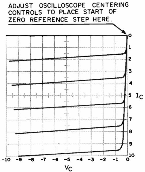
ADJUST OSCILLOSCOPE CENTERING CONTROLS TO PLACE START OF ZERO REFERENCE STEP HERE.
