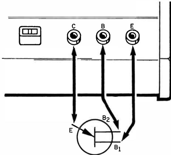
Figure 31. Set-Up and Typical Display of Unijunction Transistors
