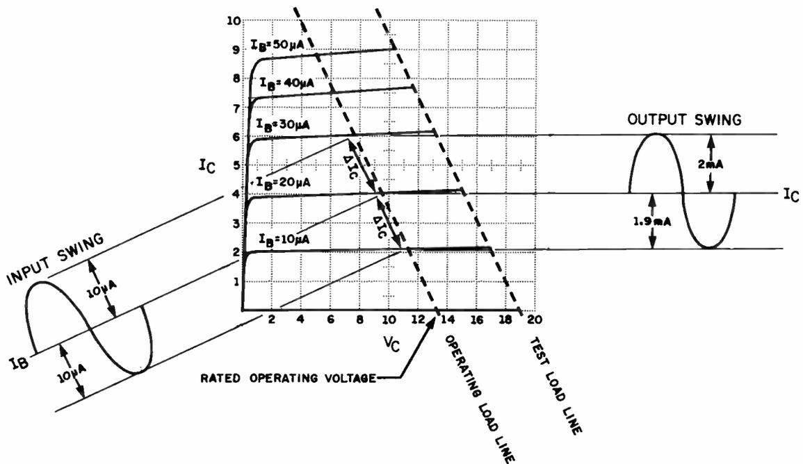
Figure 20. Measuring Current Gain Non-Linearity
