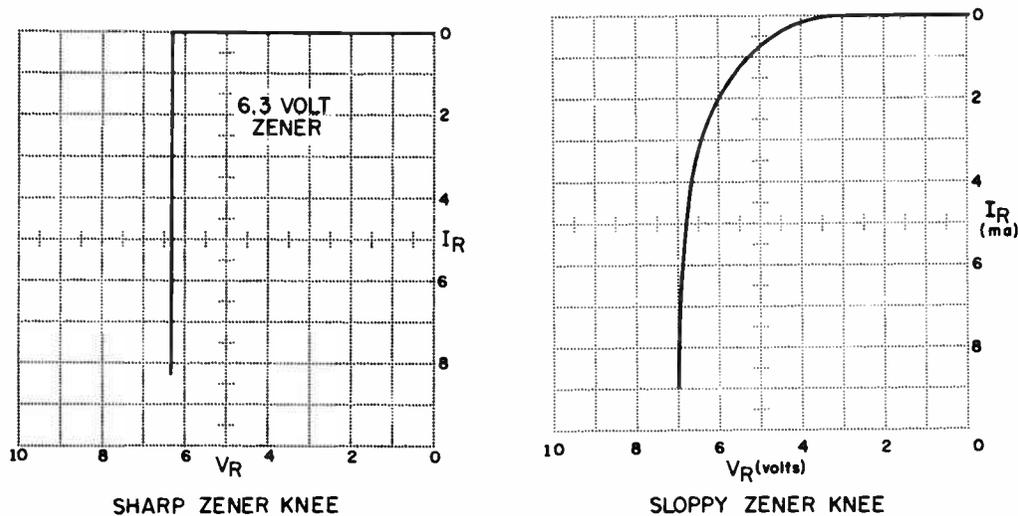
Figure 30. Typical Zener Diode Curves
