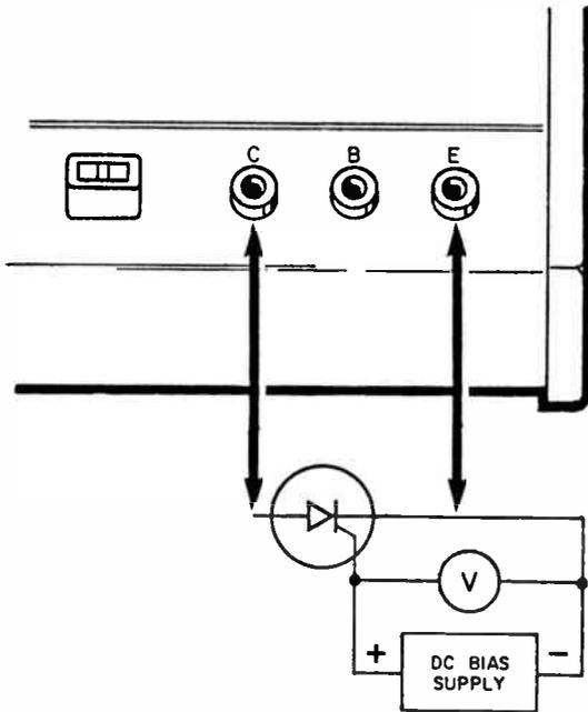
Figure 35. Testing Gate Trigger Voltage of SCR's
