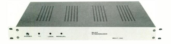
The purpose of the Pilot Synchronizer is to phase lock one or more FM exciters to a common reference using the 19 KHz pilot tone on a multiplex FM signal.
