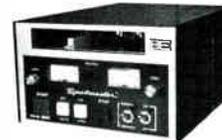
Model 3200 stereo record/playback with optional fast forward, secondary cue tone (150 Hz) and tertiary cue tone (8 KHz).
