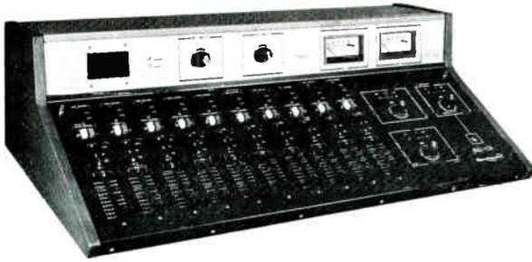
The 3006 Series Consoles bring economy to the once very expensive slide-type mixer consoles. Ten slide mixers may be switched to either of two output circuits. These assignments are made by pushbuttons, and either or both may be fed simultaneously by each mixer. A lever switch located above each mixer selects the mode of that mixer channel. When placed in the "Pgm" mode, that mixer will feed whichever output assignment the operator had selected.
