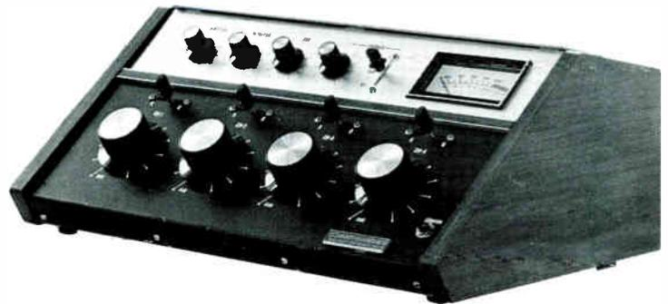
The monaural 4BEM-50 is a complete small console ideal for production, on-air, educational, or CATV use. The 4 mixers each accept two switch selectable inputs for a total of eight. Each mixer preamplifier can be wired for either microphone or line level sources. The mixers are long-life, sealed units for quiet, trouble-free operation. Speaker and headphone amplifiers are built-in for monitoring the console output, an
