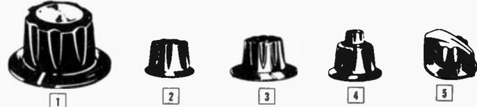
Dress up knobs for panels and equipment. Precision molded of tough black plastic, gloss finished. All have 1/4" hole and set screw. Figure 1 has spun silver inlay. Figure 3 for dual shaft concentric controls. Has white filled pointer line.
