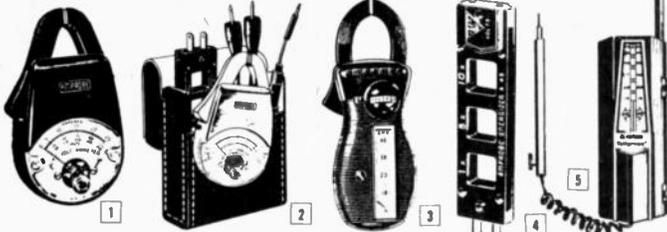
Snap around type Volt-Ammeter. Close the probe jaws around conductor of the circuit under test and read current directly on meter scale. Voltage checks are made by the use of safety type leads. It is possible to safely and accurately determine load condition of equipment without shut down.
