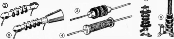
A wide selection of popular RF Chokes for receiver and transmitter circuits. R100-300 are wound on ceramic forms, R33 and R50 on molded phenolic. R175A rated 4000 volts, for 6 through 80 meters, 3000 V. Modulated. Current rating below is 20 degrees rise.
