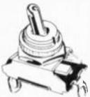
Type 125RB. 3 amps at 125 volts AC. Solder terminals. Threaded stem diameter 1/8". Stem length 1/2". Has bat handle length 3/8". Body 1/2" L. x 1/8" W. With hex and knurled nuts. Wt. 2 oz.
