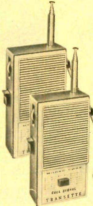
Features include: 4 transistor super regenerative receiver with volume control, crystal controlled transmitter with channel 14 (27, 125 MHz) crystal, 42" 9-section telescoping antenna and standard 9 V. transistor battery. In addition to regular voice communication the unit can transmit a code signal by "keying" the code button. Has Morse Code alphabet printed on front of unit.
