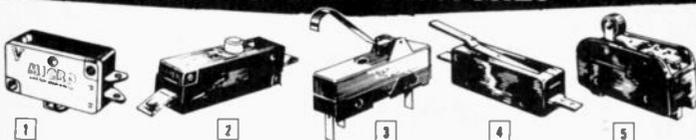
(1) Miniature Micro V-3, SPDT 10 amps @ 125 or 250 V. 1 1/2 x 1/2 x 1 1/2". Insulated plunger travels .047", O.T. .031". Wt. 2 ozs.
