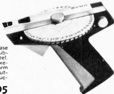
Prints both upper case and lower case (.205") letters plus regular and subscript numbers on one universal wheel. Uses 1/2" or 3/8" tape. Features "Executive" letter spacing for uniform type-set look. Automatic pull tab cutoff. Light weight all metal construction. Baked enamel finish.
