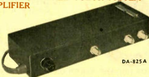
Extremely flat +25 db gain on all channels 2-83. System can't become obsolete when new channels come on the air. Ultra-low noise figure insures clear, snow-free color and black and white. Can be used with 82 channel antenna or separate VHF and UHF antennas. Long life, low cost operation. 117 V. AC. (VTF-73 or VTS-73 line tapoffs recommended). Shpg. wt. 3 lbs. Mfg. List \$64.15
