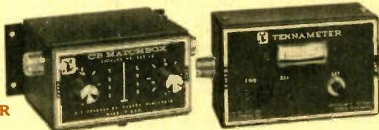
**NEW JOHNSON CB MATCHBOX.** Connects between transceiver and coax feed line to antenna. Corrects impedance mis-match, eliminates standing waves, improves performance of equipment. Handles up to 15 watts power. 4 x 3 1/4 x 2 3/8". No. 10A3004. Wt. 3 lbs.
