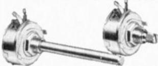
Packs 5-watt capacity into a 2 watt size unit; linear taper, 1 1/2" dia. x 3/4" deep. Model WN has full round aluminum shaft 1/4" dia. x 3" long. Model WN has fingertip knurled, slotted shaft 1/4" dia. x 3/4" long. Linear taper. Break-down, 900 V. AC rms to ground. WN or WW prefix indicates manufacturers number. Shpg. wt. 4 ozs.
