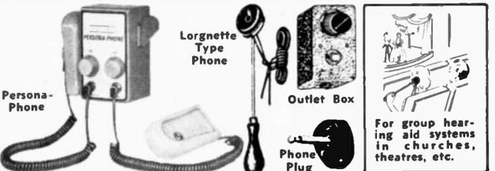
"Telex" Persona-Phone. Private listening device for church, library, museum, theatres, exhibits, etc. Small molded plastic housing contains matching transformer, 2 volume controls, 2 jacks for earphones. New sanitary acoustic shell phone units fit over either ear. Operates on 8 ohm, 70 volt or 25 volt program source. With 2 phones. Neutral tan color, gold front.
