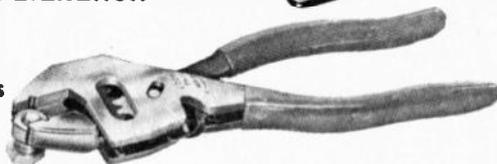
Parallel jaws give firm grip on round or flat objects. 10 to one gear ratio gives the user's hands the equivalent of 1 ton of gripping power. Extra long double-tapered jaws reach deeply into hard-to-get-at places. Extremely powerful, yet delicate enough to use on polished fittings without causing damage. Has wire cutter for large wire. Comfortable cushion grip handles, precision built, drop forged heat treated steel 8 1/2" long. No. 37A831. 86070. Plierench in pouch. **\$6.35**
