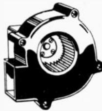
Small size, high output approx. 50 CFM. Has molded nylon blower wheel 2" dia., 1" wide. Molded housing has 1 1/2" dia. air inlet, 1/4 x 1 1/4" outlet. Powered by Howard Ind. motor rated 16 W. .003 HP, 115 V. 60 Hz AC. Overall size 4 3/4" max. dia., 3" deep. No. 18A1440. \$6.95 While Supply Lasts.
