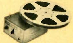
Meets the requirements of the industrial user. Erases video and audio from magnetic tapes up to 1" wide in one operation. Will also erase 2" tapes by processing one side, then turning over for second side. Has safety overheat indicator, fused circuits, heavy-duty switches and power cord. Designed for 5 min. on/15 min. off duty cycle. Size: 3 3/4" x 6" x 8". For 10 V. 50-60 cy. AC. Shpg. wt. 8 lbs. Mfg. list, \$100.00.
