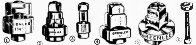
Quickly cuts clean, accurate holes in chassis or panel to accommodate sockets, switches, controls, meters, etc. Cutting is done by 2-point punch driven by 3/8" dia. square head cap screw. Operates simply with an ordinary wrench.
