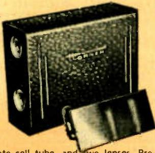
Compact single unit with exciter lamp, photo-cell tube, and two lenses. Projects a beam of light across any entrance from 3 to 20 ft. in daylight. Mirror reflects beam back into photocell. Breaking of this beam by any person or moving object operates built-in relay which in turn sounds chime furnished. Perfect for professional offices, stores, factories, homes—anywhere. Grey hammertone metal case, size only 8 3/8 x 6 1/2 x 2 5/8". For 115 volts, 60 cy. AC. Shpg. wt. 8 lbs.
