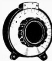
Planetary drive ratio 8 to 1 in 180° counter clockwise. Brushed silver dial with deep-etched black-filled markings reads 0 to 100. Knob and housing molded black phenolic. Surface mounting for 1/4" shaft. Shpg. wt. 8 oz.
