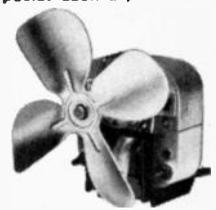
Quiet operating, compact balanced assembly especially well suited for cooling tubes and equipment. Can be mounted right on the chassis with other parts. Powered by high quality continuous duty shaded pole motor equipped with bronze oilite bearings, 1/4" shaft. With four blade Torrington impeller. Size 2 1/2" W. 3" H. 3" deep. For 115 V. 60 cy. AC. No. 18A1353 Special Each \$2.49 10 @ \$2.19 Each
