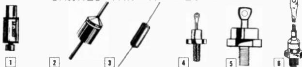
Dimensions: Fig. 1 overall  $\frac{3}{8}$ " dia. x 1" L.; Fig. 2 Body  $.195$ " dia. x  $.335$ " L.; Fig. 3 Body  $.125$ " dia. x  $.342$ " L.; Fig. 4 10-32 Stud x  $1.25$ " overall length; Fig. 5  $\frac{1}{4}$ -28 stud x  $1.435$ " overall length; Fig. 6  $\frac{3}{4}$ -16 Stud x  $6\frac{1}{4}$ " overall length.
