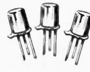
3 200 MC Silicon Epitaxial Transistors. Similar to 2N706. TO-18 case. Vcb 25, Hfe 20, 10 MA. 20A1105. 3 For ..... 99c
