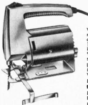
Well balanced. Crosscuts, rips, scrolls, notches its own starting hole. Clears cutting line with air stream. 3 amp 115 volt AC motor develops 3/4 HP industrial rating. Capacity 2 1/4" at 90° 1 1/8" at 45°. 3/8" stroke. 300 strokes per minute.
