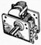
2 Variable 2-Gang Capacitors. 1 with 280-10 mmfd RF, 100-6 mmfd osc. section; 1 with 135-10 mmfd RF, 90-6 mmfd. osc. section.
