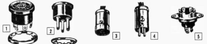
Any plug in this group mates with any socket with same number of pins. 78 series mount in 5/8" hole with push-on spring ring. Can be chassis mounted or wired to cable. 7-pin sockets fit 7-pin miniature tubes. Avg. shpg. wt. 5 ozs. per 20. Fig. ③ and ④ are 5/8" dia., 1 1/2" long cadmium plated brass. Fig. ⑤ is shielded chassis socket. Avg. shpg. wt. 1/2 ozs.
