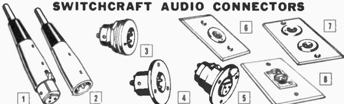
Interchangeable with Canon XLR-3, XLR-4 and Amphenol 91-850 series. Professional style audio connectors made for rugged service. Connectors are polarized with exclusive grounding lug on all units. Shells are made of die-cast zinc, satin nickel finish. Inserts are of high-impact plastic. Wall plates are brushed stainless steel and fit standard electrical outlet boxes.
