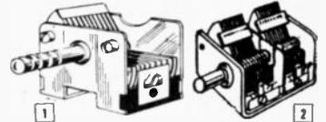
(1) SEMI-MIDGET 365 MMF. All brass and aluminum construction with smooth action ball bearings. 1/4" x 1 1/8" long shaft. Panel or base mount. 1 3/8" W. x 1 3/8" H. x 1 3/8" D. Import. **No. 12A2462. Each 79c** 10 Lots **71c** Each
