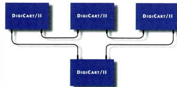
D-NET File Transfer Network, shown in a typical configuration.
