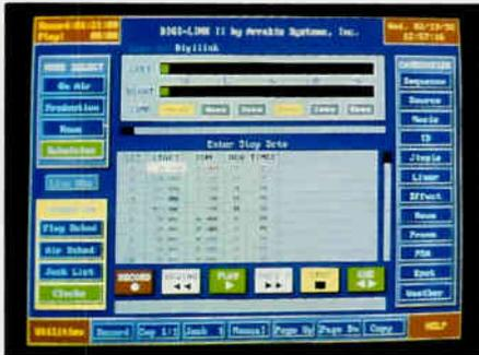
Under the 'Air Schedule' button, the announcer and type of hour are chosen. Any of up to 40 announcers are available. Each hour may be selected for satellite, live assist, manual, or full automation operation.
