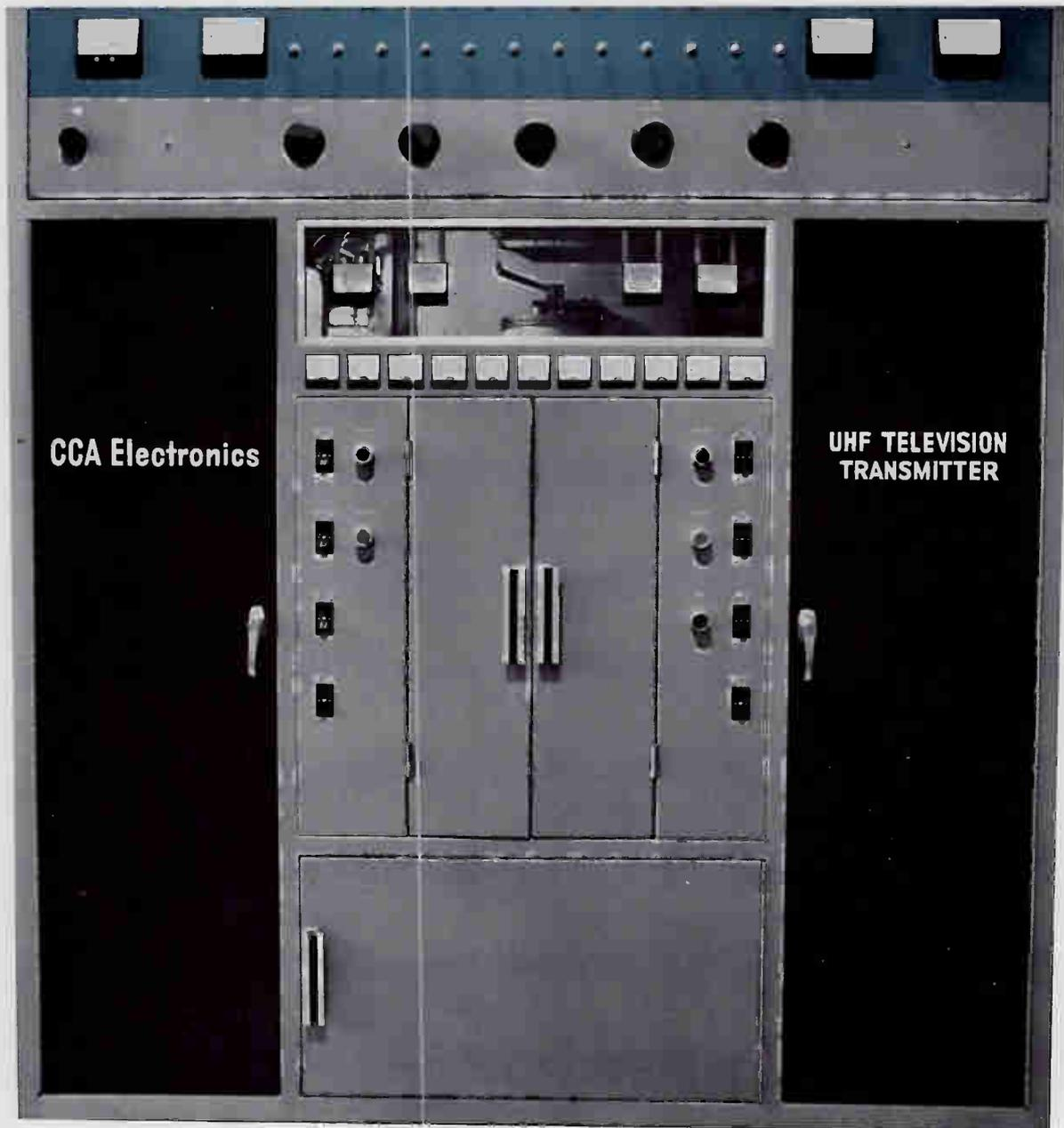
The CCA RF Driver contains two independent solid state exciters one for the aural the other for the visual. The output of the aural exciter is 10 watts. Substantially more than the 2 watts required to drive the aural klystron. The Visual exciter drives a YD 1270 triode which can conservatively produce 25 watts. This stage
