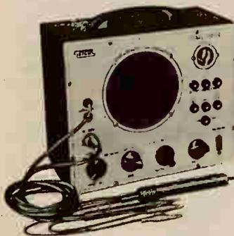
Two separate input channels assure maximum applicability to both RF and audio work. Magic eye tube and speaker provide both visual and aural signal monitoring. Calibrated wattmeter to measure power consumption of equipment being tested. Output for VTVM or oscilloscope. Built-in transformer or speaker may be used as substitutes for suspected components in defective equipment. Complete with shielded RF crystal demodulator and direct probes.
