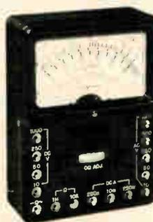
This pocket portable is a versatile general utility instrument. Make readings easily on all 14 ranges. Large meter face. High-impact plastic case. DC VOLTAGE: 0-10, 50, 250, 1000 volts. AC VOLTAGE: 0-10, 50, 250, 500, 1000 volts. DC CURRENT: 0-250 $\mu$ A, 10mA, 250mA. RESISTANCE: 0-20K, 2 Meg. DECIBELS: -20 to +62 db. ACCURACY: DC  $\pm 3\%$ , AC  $\pm 4\%$  of full scale. SENSITIVITY: 4000 $\Omega$ /V DC; 2000 $\Omega$ /V AC. SIZE: 4 $\frac{1}{2}$ "H x 3 $\frac{3}{8}$ "W x 1 $\frac{1}{8}$ "D.
