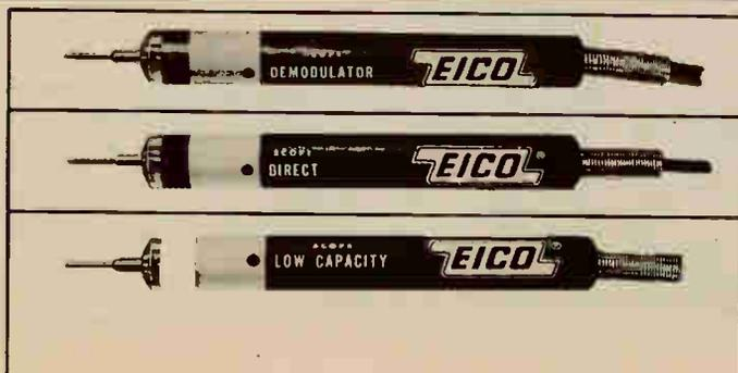
**PSD 'Scope Demodulator Probe** For signal tracing and checking of TV/radio RF and IF stages. Permits scope to be used as waveform tracer, gain analyzer and alignment indicator in all stages. Demodulates AM carriers between 150 kHz and 250 MHz. **Kit Assembled**
