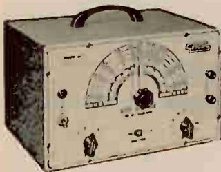
Fills requirements of audio engineer, technician and hobbyist. Frequency range: 20-200,000 Hz on sine wave, 60-30,000 Hz square wave. Output voltage: 10 V across 100 ohms. Distortion: less than 1%. Because the output is constant over a wide frequency range, the distortion is low and the square wave has a good rise time.
