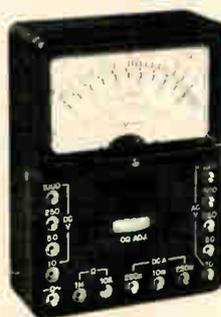
This pocket portable is a versatile general utility instrument. Make readings easily on all 14 ranges. Large meter face. High-impact plastic case. DC VOLTAGE: 0-10, 50, 250, 1000 volts. AC VOLTAGE: 0-10, 50, 250, 500, 1000 volts. DC CURRENT: 0-250 $\mu$ A, 10mA, 250mA. RESISTANCE: 0-20K, 2 Meg. DECIBELS: -20 to +62 db. ACCURACY: DC  $\pm 3\%$ , AC  $\pm 4\%$  of full scale. SENSITIVITY: 4000 $\Omega$ /V DC; 2000 $\Omega$ /V AC. SIZE: 4 $\frac{1}{4}$ "H x 3 $\frac{3}{8}$ "W x 1 $\frac{1}{8}$ "D.
