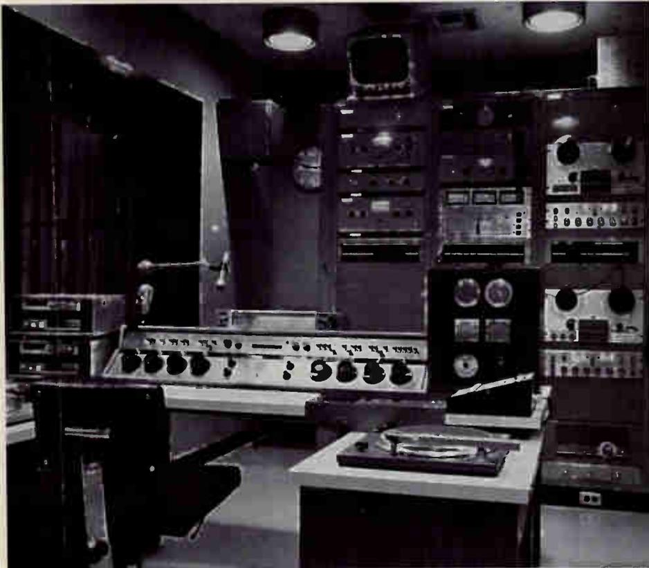
Most of the live studio shows at WSIE originate here, in the main control room. Shown in the foreground are the Gates' 8-channel mono/stereo Dualux II audio console, Criterion record/playback system and CB-77 turntable.
