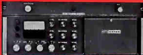
**Operating Controls**—The local control panel, with master blanking and iris (servo) controls is at top. The camera control unit is below, showing the null meter for simple daily checkout of black and white levels on each channel.
