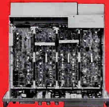
**Maximum Access**—The camera control unit extends out on its rack slides, and may be swung up on for 90-degree presentation and immediate access to either the top circuit boards (shown), or those on the bottom.
