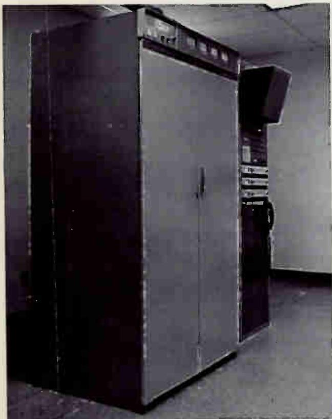
The Gates FM-10H transmitter, and a five-bay directional FM antenna array (also supplied by Gates), provide WSIE a 50,000-watt stereo signal.
