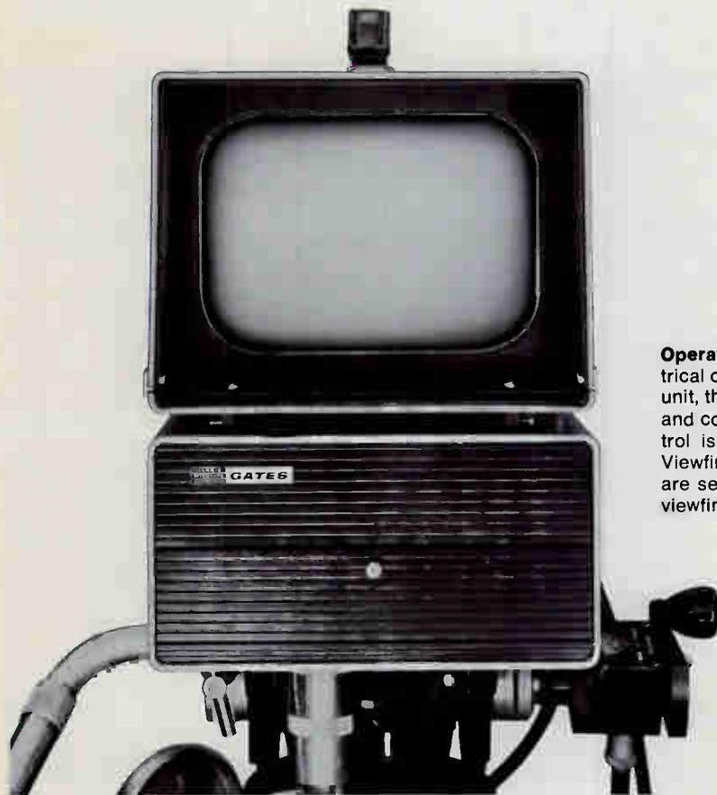
**Operating Simplicity**—With all TE-201 electrical operating controls at the camera control unit, the cameraman has only to frame, focus, and compose the picture. The zoom lens control is at right, the focusing control at left. Viewfinder brightness and contrast controls are set in under the viewfinder. At top is the viewfinder carrying handle.
