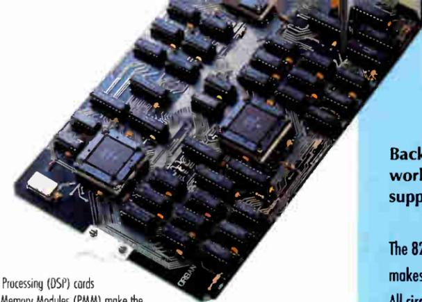
Digital Signal Processing (DSP) cards and Program Memory Modules (PMM) make the 8200 fully expandable. By installing new boards and modules, future software upgrades and processing structures can be added easily—without purchasing a new box!
