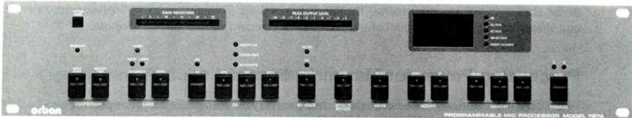
Three-band parametric equalizer, compressor, de-esser, noise gate, and compressor gate integrated in a compact, powerful system. Stores up to 32 different control setups in memory for instant recall. Designed for mic processing and voice recording, but versatile enough for many other production uses. Optional MIDI interface.
