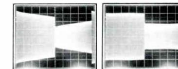
WITHOUT TILT CORRECTION WITH TILT CORRECTION
