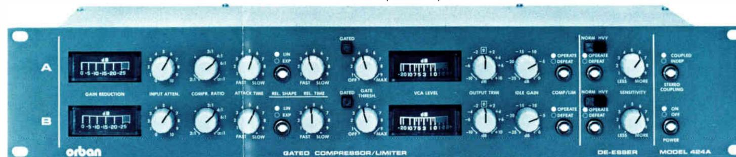
The defeatable silence gate (controlled by the front-panel GATE THRESHOLD control) avoids noise rush-up during near-silent passages by radically slowing the release process, thereby forcing the VCA gain to freeze and then to move very slowly toward the average of the last 30 seconds of gain reduction. (This is an automatic "idle gain" function, similar to the manually set IDLE GAIN on our 424A Gated Compressor/Limiter/De-Esser.)
