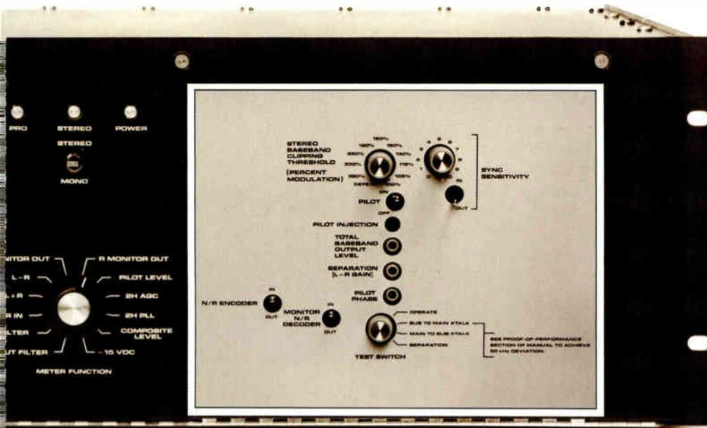
FRONT DOOR REMOVED SHOWING SETUP CONTROLS
