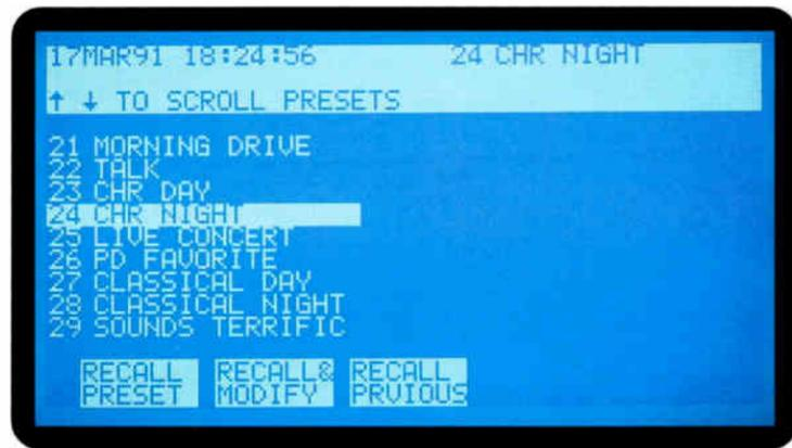
RECALL any one of the factory installed or station installed presets. They can be recalled from the front panel or from a local or remote computer. Or they can be automatically recalled on a programmed schedule.
