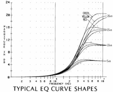
There are no superfluous equalization controls which might be claimed to add "versatility", but which are in fact easy to misadjust. All of our curve families are scientifically correct in the sense that they match the "average" receiver in the midrange and therefore cannot create a "honky", fatiguing lower-midrange boost.
