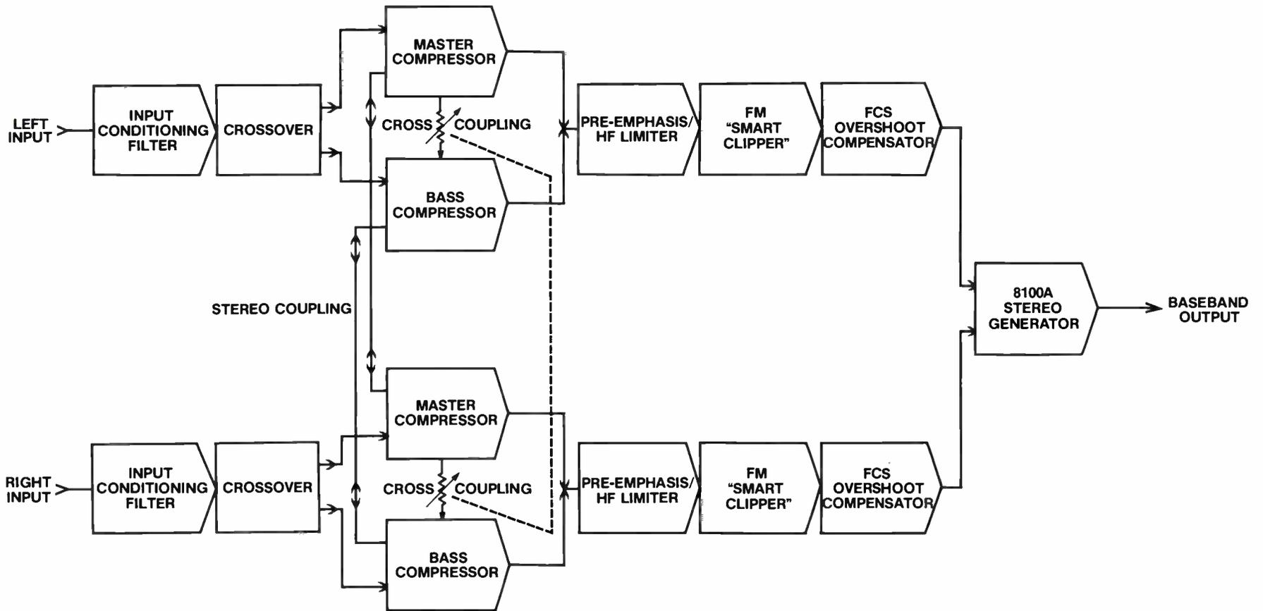
**OPTIMOD-FM MODEL 8100A SIGNAL FLOW DIAGRAM**
