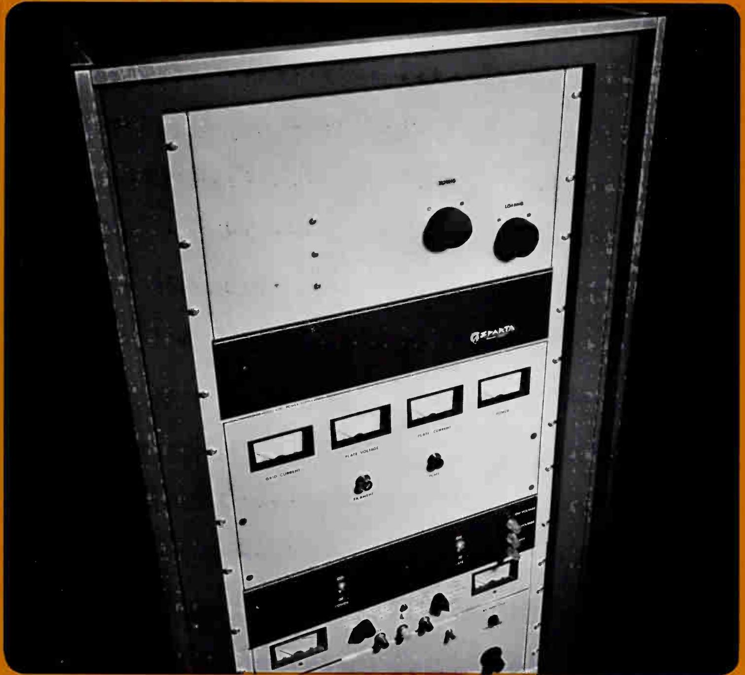
SPARTA'S Model 600 FM Transmitter for standby or low power operation offers the buyer a choice of tube-type or solid state exciters. The low-profile 250 watt unit ties the chosen exciter to a single 4CX350A tetrode, accomplishing a top quality FM signal with minimum cost in space, maintenance, complexity or dollars. All power supplies are solid state. And keep in mind that the entire self-contained unit is only four feet seven inches high!
