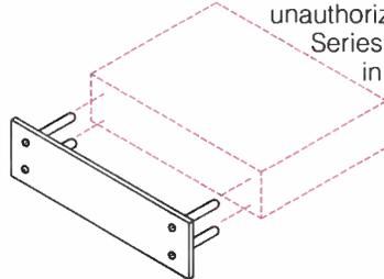
**PS-2 Power Supply** Replacement for power supplies originally included with SX200 Series, products sold in North America. Input 120VAC, output 16 volts, AC, 10VA.
