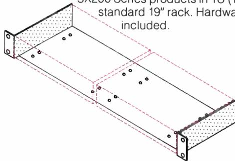
**SR-4 Stack Rack** Optional accessory rack provides "stack" mounting for four SX200 Series products. Hardware included.
