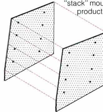
**SC-2 Security Cover** Optional accessory cover prevents unauthorized adjustment of SX200 Series products when mounted in RM-2 or SR-4. Hardware included.
