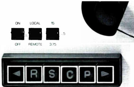
illumination of the transport controls simplifies operation with the activated button glowing brighter than the others. A flashing record light indicates when the record electronics are ready. Pushing the record and play buttons simultaneously puts the machine in record and the record indicator light then glows steady. For added versatility all 1400 models feature a three speed (3-3/4, 7-1/2, 15 ips) drive system.
