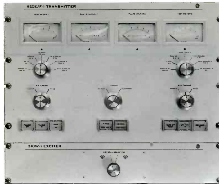
Extended metering/control panel and crystal oscillator exciter
