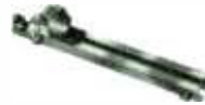
SPRING HANGER. ANDREW 14379. Use at 50 ft. intervals. Accommodates line expansion. Mounts through 3/16" diameter hole or adaptors. Part No. 124 0032 189
