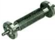
FLEXIBLE SECTION. ANDREW 20695. Accommodates vibration and angles up to 30 degrees. Maximum offset is 1/4". Length 10". Part No. 099 0434 000
