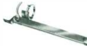
SPRING HANGER. ANDREW 13925. Use at 10 ft. intervals. Accommodates line expansion. Mounts through \frac{1}{8} " diameter hole or adaptors. Part No. 097 6122 000
