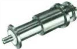
BREAKAWAY SECTION. ANDREW 2962. Permits easy opening of transmission line run. Pressure tight when closed. Length, 19 \frac{1}{16} ". Part No. 099 0442 000
