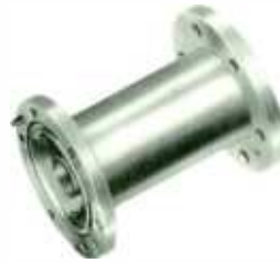
ADAPTOR, male to male (3/8" EIA), use between fittings with fixed male inner connectors. 50 ohm—TYPE 23187. 75 ohm—TYPE 24530. Part No. 097 7262 000-23187
