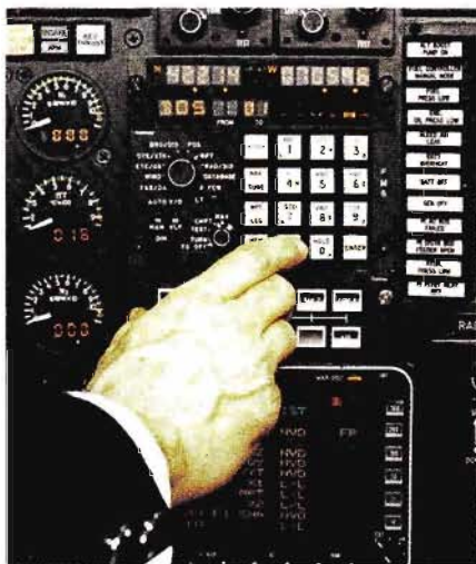
The advanced Collins flight management system (FMS-90) is used to program automatic navigation on board the aircraft, and can control several other avionics systems. 1981 photo.
