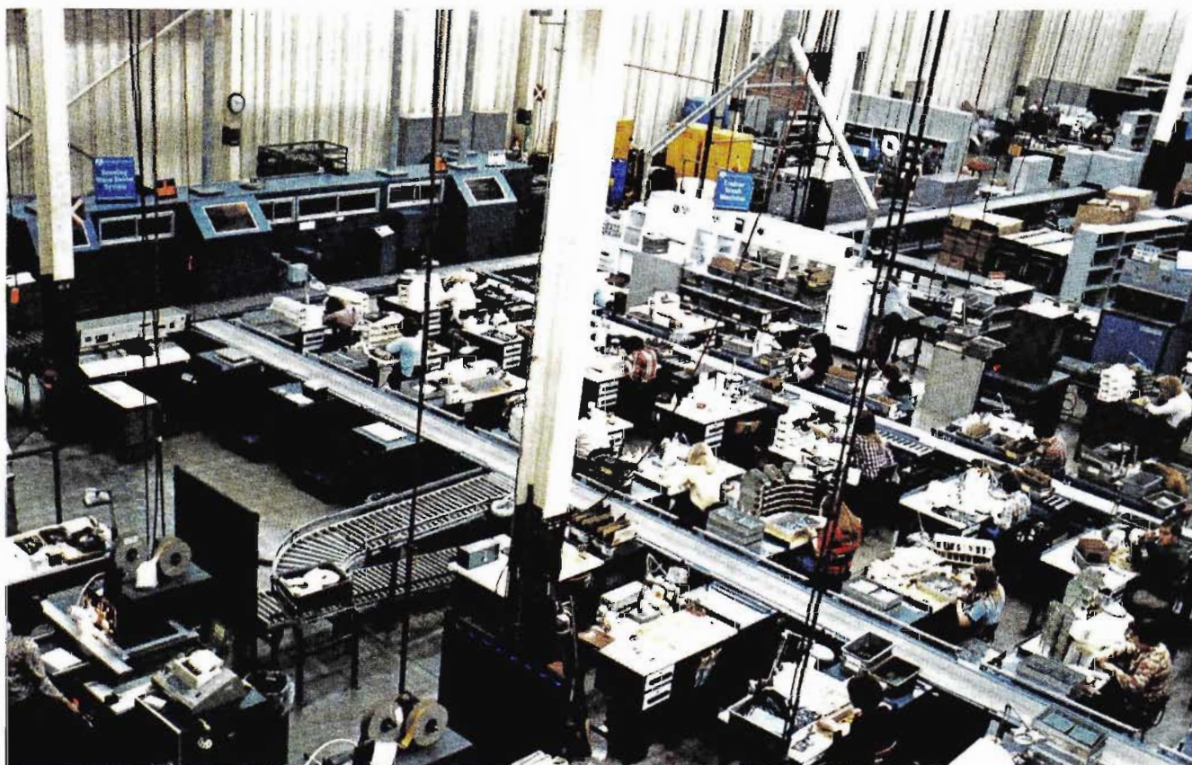
Collins Air Transport Division Process Center employs advanced automatic component insertion, wave solder, wash, test and conformal coating techniques to produce multilayer circuit boards.
