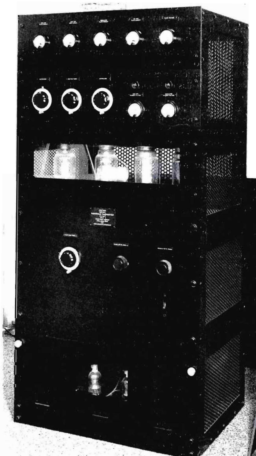
The large 20B transmitter used by the Byrd expedition was designed primarily as a broadcast transmitter, although some amateur operators who wanted maximum power also used it.
