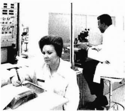
MOS chips were electrically tested by computer-generated test sequences at the Newport Beach facility. Operator is Erna Sanches. Lab technician is Chester Bishop.
