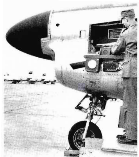
Installation of a Collins ARC-27 radio in an F-86 fighter jet.
