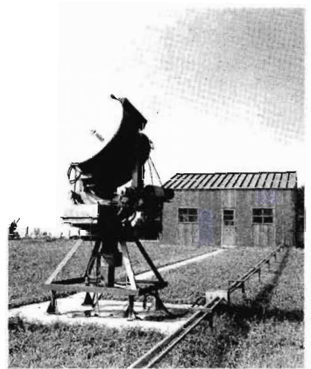
An early version of the Collins radio sextant, at the Feather Ridge Observatory.
