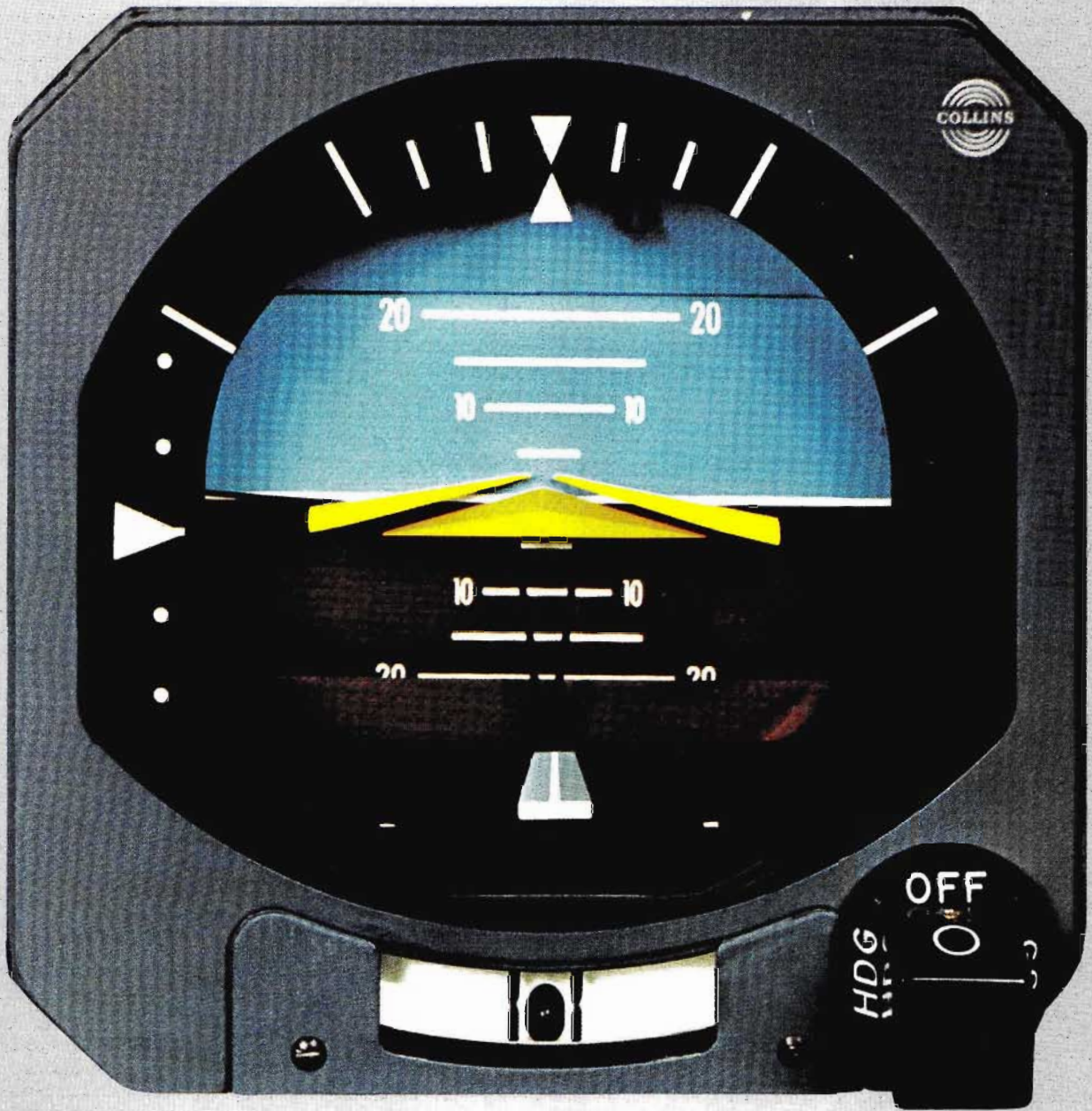
The "V-bar" indicator gave pilots a new way to view flight information.
