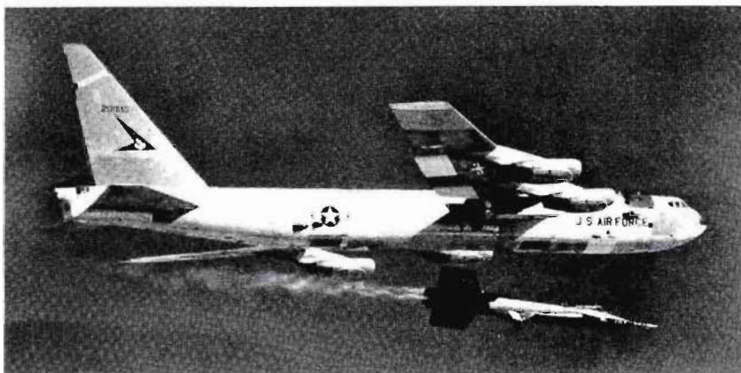
Dropped from the wing of a B-52, the X-15 used rocket power to accelerate to speeds of more than 3,600 miles per hour.
