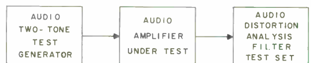
Figure 8-13. Test of Intermodulation in Audio Amplifier
