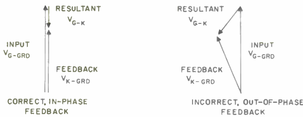
Figure 7-13. Vector Relationship of Voltages for Two-Stage Feedback
