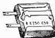
Contact cooled rectifier
