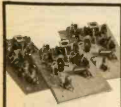
"Drop-In" Interchangeable Front End Modules For Converting the DigI Scan-8 to either Low VHF/FM, High VHF/FM, or UHF/FM.
