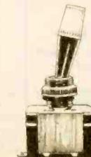
Snap action. Lamp built into handle. End of handle lights in "on" position. Large  $1\frac{1}{4}$ "-long bat handle. Bushing  $\frac{1}{2} \times \frac{1}{8}$ ". Solder lug terminals. Contacts rated at 10 amps @ 125 VAC. Size.  $\frac{5}{8} \times 1\frac{1}{8} \times \frac{3}{8}$ ". 275-670. Ship. wt. 3 oz. ....2.19
