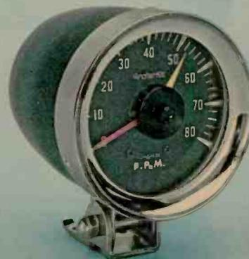
For any 12-volt system. Reads 0-8000 rpm. Accuracy, ±2%. Deflection angle, 240°. Shock/vibration resistant. 3¼" illuminated dial.
