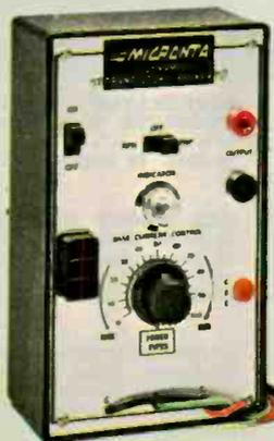
Shows electrode open and short circuits, current gain. Permits matching of similar transistors in operating circuits. GO/NO GO test from 5-50 mA on power types. Front panel quick-check socket; clip leads for "in-circuit" test. 6 1/4 x 3 x 2 1/2".
