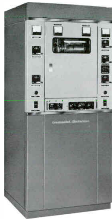
Type 414D 1,000 watt AM short wave transmitter
