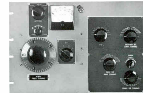
Variable Frequency Oscillator For MF Broadcast Transmitter
