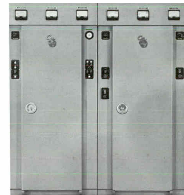
Type 415B/416B 5,000/10,000 watt AM short wave transmitter
