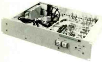
The combiner control unit provides all interlock and sequencing functions. It is designed to fit on the control panel furnished with the 817R-1 transmitter.
