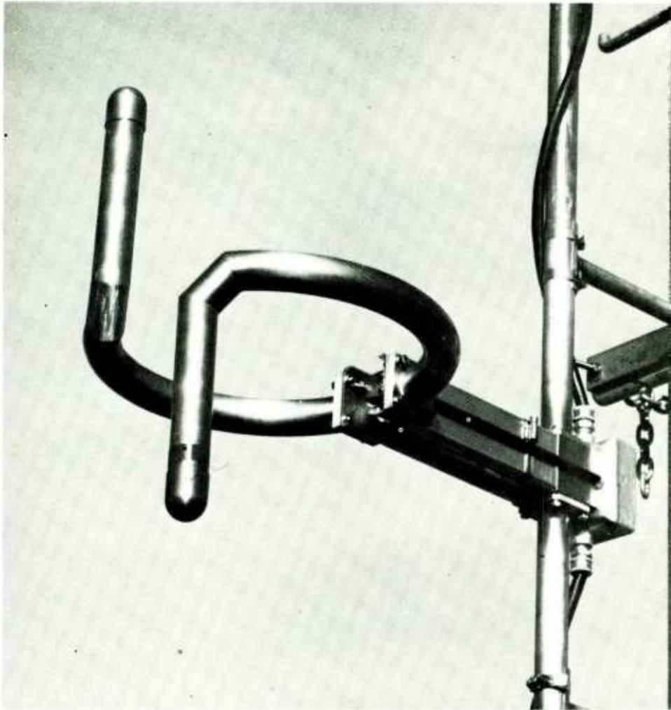
The rings of the antenna are mounted on 1 $\frac{5}{8}$ " line and are end fed. A 6 ft. matching transformer extends below the lower bay and terminates in a 1 $\frac{5}{8}$ " EIA, 50-ohm flange.
