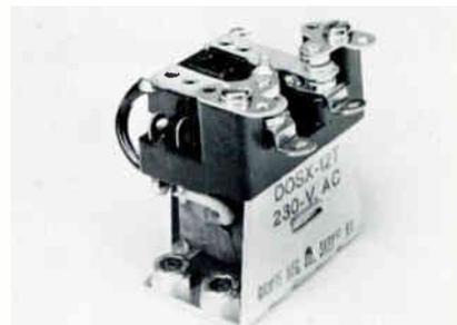
DOSX-7T: 115 vac coil, DPDT 15 amp, 115 vac non-inductive contacts. DOSX-12T: same as DOSX-7, except with 230 vac coil. DOSX-59T: same as DOSX-7, but has 110 vdc coil.
