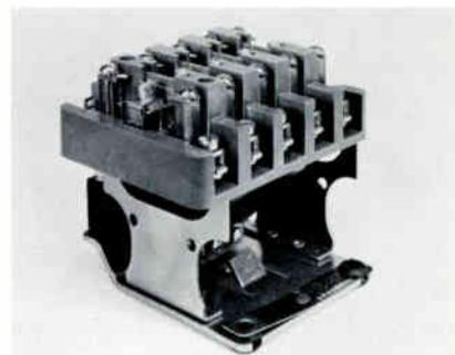
**RBM CONTACTORS.** Heavy-duty, industrial contactors, they may be connected at TRC-T switching output to control external pushbutton circuit, or for interlocking use in external circuitry. Recommended for Plate on-off control. RBM 101130-101: 115 vac coil, 3 PNO reversible contacts, rated 10 amps, 115 v ac non-inductive. RBM 101150-101: same as RBM 101130-101 but has 5PNO reversible contacts. RBM Contactors also available with 230 vac coils, and with 15 amp reversible and 25 amp N.O. contacts.
