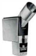
**SSP10** Decorative stand adapter. Connects directly to each basic microphone module. Includes on-off switch and receptacle for CA10, Cannon XLR-3-11C plug, or Amphenol 91-854. Permits tilting the microphone through a 90° arc. Mounts to any stand with standard 5/8-27 NPSM thread. Size: 3-7/16" x 2 3/4" x 1 1/8". Weight: 1/2 lb.
