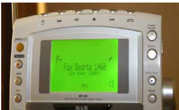
Figure 5.4: Live screen-shot of DRM receiver in AM mode displaying AM service name
