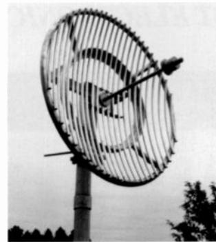
**Grid Parabolic Antennas**
