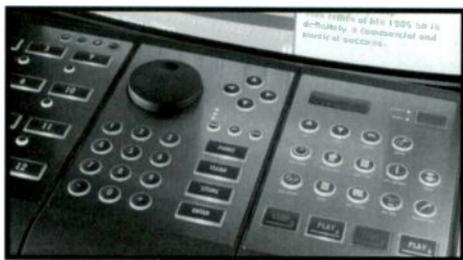
Modular control panels provide intuitive, direct control of an entire range of station operations from recording, to editing, to broadcast. Each user plugs in as many modules as they need with a single serial port connection.
