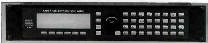
ware is simple to understand, and gives your station the flexibility of using RBDS for changing data. The SC-100 includes an RS-232/modem Interface for easy connection.
