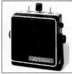
(300Hz to 10kHz) output from the internal speaker and a full ten octave (20Hz to 20kHz) output from a line level phone jack. A switchable pulse generator can be used to interrupt the noise output every four seconds. The NG-1 is powered by an internal nine volt battery or AC power. A handy mounting bracket is provided for using the NG-1 in fixed installations for noise masking.
