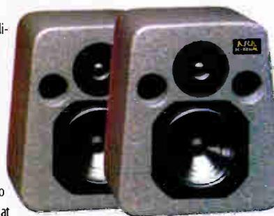
The KRK **RoKIT** speaker offers a completely shielded monitor designed for lower power applications. Built into a KRK unclosed linear enclosure the RoKIT features a 1" Silk Dome Tweeter and a 6.5" Long Stroke Polyvinyl Woofer. The RoKIT's frequency response is a wide range 69Hz–24kHz ±2dB and can output a Maximum SPL of 104dB. With nominal impedance of 8 Ohms, these nearfield monitors are rated at 75 watts.
