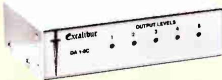
Optional rack ears mount either DA in one RU. S/N >80dB at unity gain, input common mode rejection is greater than 75dB at 1kHz, and THD is less than 0.01%. Maximum gain is 18dB and maximum input and output levels are +22dBm.
