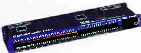
Relays are magnetic latching. Each relay can be set, cleared, or activated momentarily. The DT-55 can also act in an interlocking mode: when a button is pressed, its associated relay is set, and all others are cleared. Tones indicate the status of the external inputs. Holes are provided for mounting to a surface or to a user-supplied, single space rack panel.
