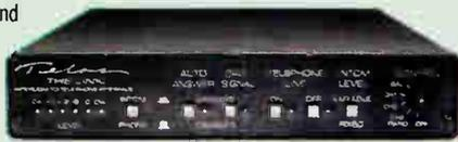
The Link allows natural, full-duplex communication without level or feedback problems, thanks to adaptive digital hybrid technology. Both the telco and comm paths use digital auto-nulling hybrids, so neither party misses a syllable. A digital audio processor performs automatic gain control, smart gain switching to enhance hybrid performance, high pass filtering to reduce hum and interference, pitch shifting for feedback reduction, and call signal generation.
