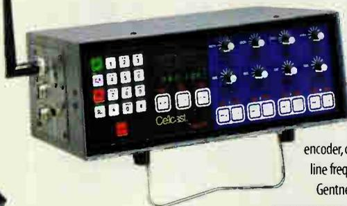
range, and its included four-channel mixer provides program and cue channels, and mic/line selectable inputs. Also included is a software selectable single line encoder, compatible with analog single line frequency extenders (Comrex, Gentner) for improved audio frequency response. A count up/down timer is
