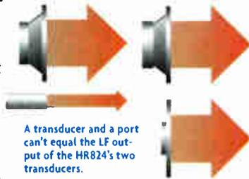
A transducer and a port can't equal the LF output of the HR824's two transducers.
