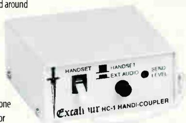
Pressing the front panel button disconnects the handset and connects the external audio in/out jacks to the telephone. Releasing the button reconnects the handset, allowing normal use of the phone. External audio is connected via separate input and output jacks. Both inputs and outputs are 1/4" TRS jacks wired so that you may use either balanced or unbalanced connectors.
