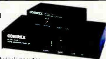
The TCB-1 Manual Coupler provides a switched hold connection. Unbalanced audio in/out is on a single 1/4" TRS connector. The unit does not require power. The TCB-2 Auto-Answer Coupler answers the telephone line on the first ring and disconnects that line when the caller hangs up. An A/C power supply is included. If your CO does not provide loop drop, order the optional dial tone detect board.
