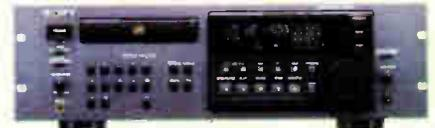
cuing by CD frame unit, with a rehearsal function. A Jog Dial precisely places the cue point, while the cue/standby button offers back cuing capability. The CDP-D500 operates with a variety of remote interface options, including RS232C, GPI, and supplied wireless remote. Word sync input is provided via BNC connector, and  $\pm 12.5\%$  varispeed may be employed in 0.1% increments.
