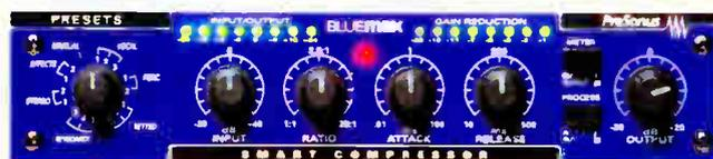
Would you believe a compressor/limiter with a brain? That's what you get with the BlueMax from PreSonus. 15 studio pre-sets and a manual mode give you full control over compression parameters including: variable I/O, attack/release times and ratios from 1:1 to 20:1. Onboard metering shows input/output levels and gain reduction for stereo and mono operations. The BlueMax takes up only 1/2 of a rack space and has an internal power supply, eliminating the need for yet another wall wart.
