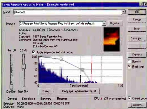
Depending on the signature applied, the Acoustic Mirror can simulate responses varying from large concert halls to the vintage sound of old tube microphones. In addition to achieving realistic imaging, the impulses can also be used to generate unique effects.
